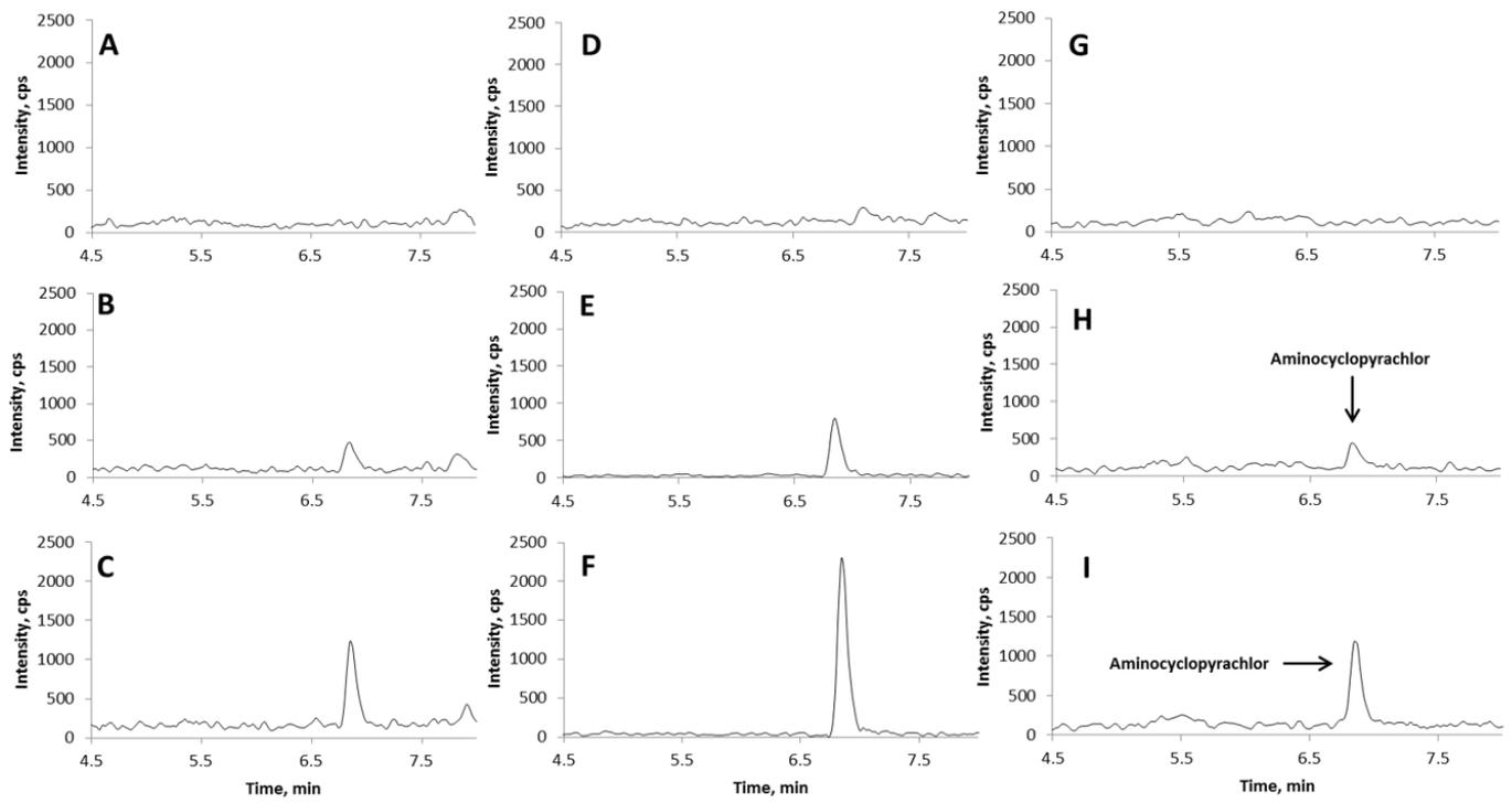
Figure 2: Chromatographs of Aminocyclopyrachlor Extracted from corn meal, soil and soy meal.
