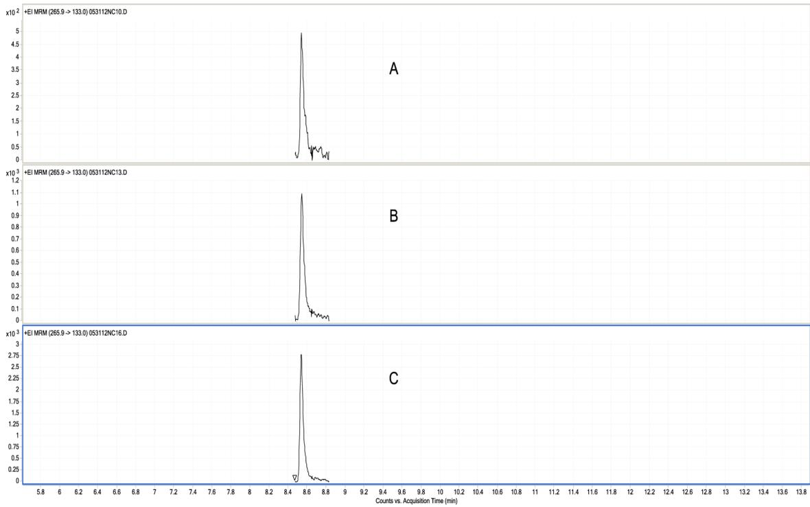
Figure 6. GC-MS/MS chromatogram (MRM) of chlorothalonil fortified in olive oil blank at 200 ng/g (A), at 500 ng/g (B), and at 1000 ng/g (C). The sample concentration is 0.0167 g/mL with 1  $\mu$ L injection volume.
