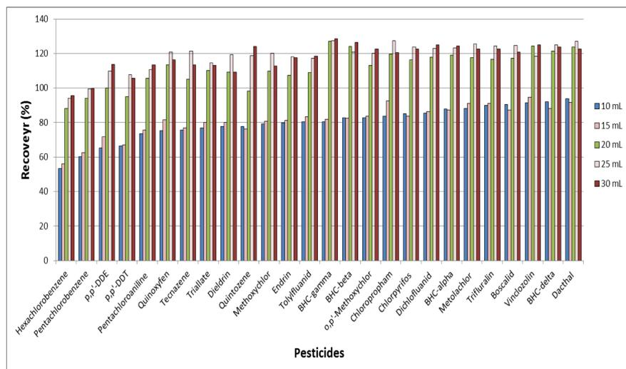
Figure 1. The response of pesticide extraction from 0.5 g of olive oil using different amount of acetonitrile and analyzed by GC-MS/MS (after matrix concentration adjustment).
