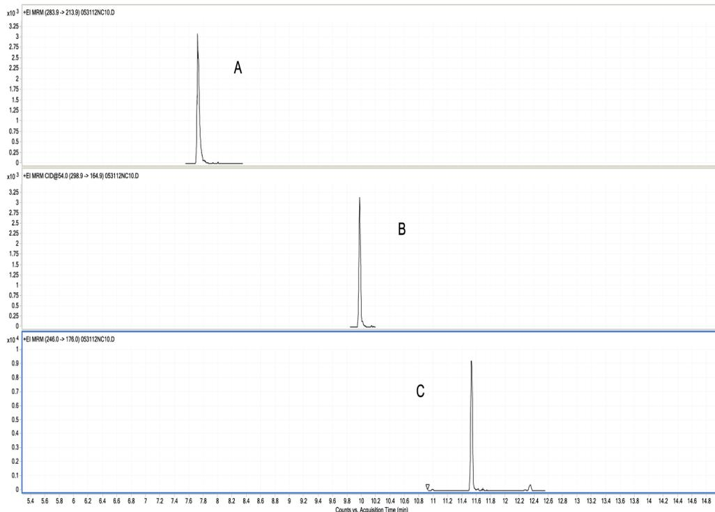
Figure 4. GC-MS/MS chromatogram (MRM) of hexachlorobenzene (A), dacthal (B), and o,p DDE (C) spiked in olive oil blank at 200 ng/g. The extract concentration is 0.0167 g/mL with 1  $\mu$ L injection volume.
