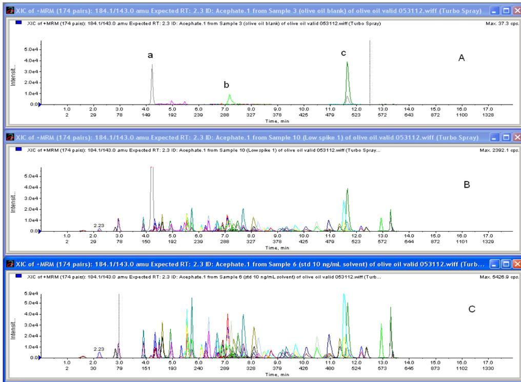
Figure 3. Reconstructed LC-MS/MS chromatogram of olive oil blank (A), olive oil blank fortified with standard mix at 200 ng/g (B), and 10 ng/mL standard mix in acetonitrile (C). The sample concentration is 0.0167 g sample/mL solvent with 1  $\mu$ L injection volume. Peak a and b are compounds found in olive oil. Peak c is d10-chlorpyrifos (internal standard).
