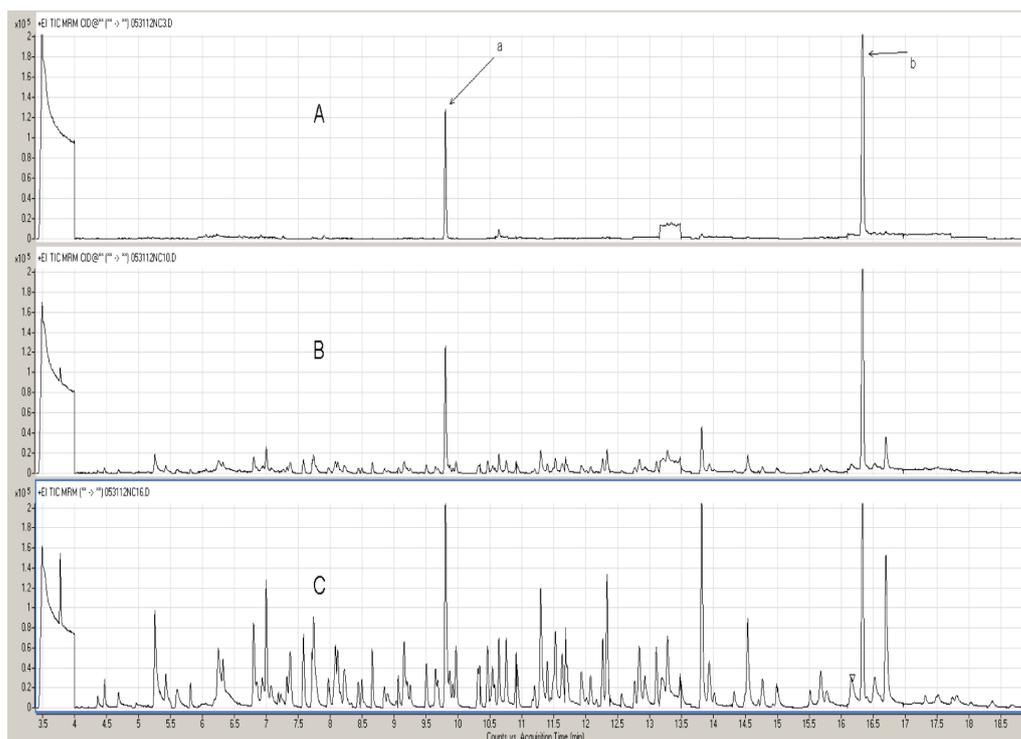
Figure 5. Reconstructed GC-MS/MS chromatograms of olive oil blank (A), olive oil blank fortified with standard mix at 200 ng/g (B), and at 1000 ng/g (C). The sample concentration is 0.0167 g/mL with 1  $\mu$ L injection volume. Peak "a" is d10-chlorpyrifos (internal standard). Peak "b" is an unknown compound found in olive oil.
