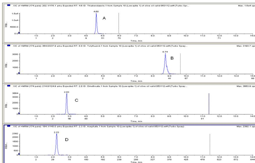
Figure 2. LC-MS/MS Chromatogram (MRM) of thiabendazole (A), tolyfluanid (B), omethoate (C), and acephate (D) spiked in blank olive oil at 200 ng/g. The sample concentration is 0.0167 g sample/mL solvent with 1  $\mu$ L injection volume.
