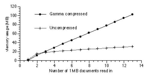
Figure 9. Memory usage for original and in-memory gamma compressed TELLTALE.
