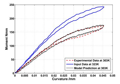
(b) Model prediction for 303K comapred with corresponding experimental results using the data at 323K as input. The average error for this case between the model predictions and experimental results was  $\sim 8\%$
