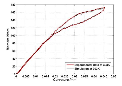
FIGURE 4 – Model prediction for the superelastic response of NiTi SMA wire at 303K. Model prediction and experimental results show a close match. The close match of simulation results shows the power of Preisach model since the Preisach parameters were chosen to fit the data. Experimental results at 303K were obtained from Rejzner et al. (2002).
