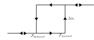
FIGURE 3 – Basic hysteretic element or hysteron used in the Preisach Model. Directions of allowed transformations are represented by the arrows on the hysteron Doraiswamy et al. (2011).
