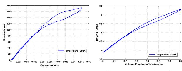
(a) Bending moment v/s curvature plot at 303K Rejzner et al. (2002).
