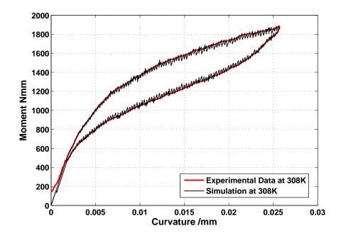
FIGURE 5 – Model prediction for the superelastic response of Cu-Zn-Al SMA beam tested at 308K showing a good match. The jaggedness in the response is due to employment of a discrete Preisach model in simulation. Experimental results at 308K were obtained from Rejzner et al. (2002).
