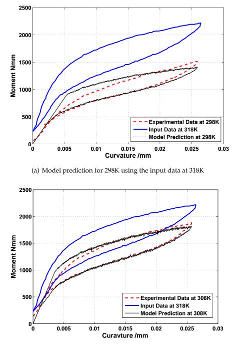
(b) Model prediction for 308K using the input data at 318K
