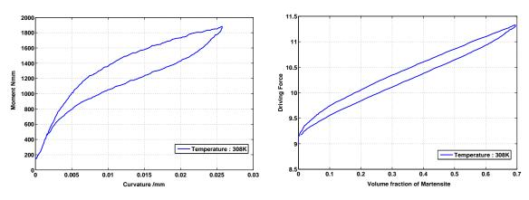
(a) Bending moment v/s curvature plot at 308K Rejzner et al. (2002).
