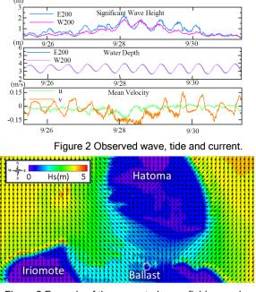
Figure 3 Example of the computed wave field around Ballast
