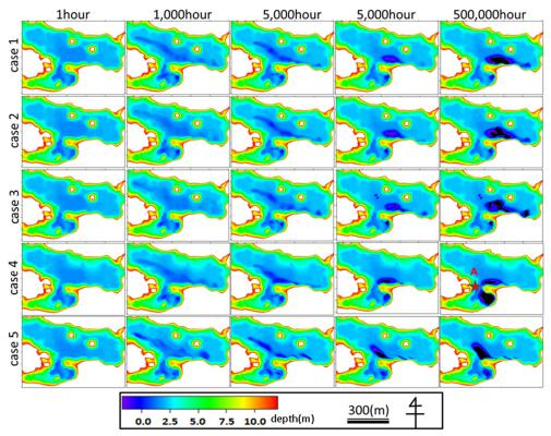
Figure 4 Time-varying computed accumulation of coral gravels in different cases 1, 4, and 5.
