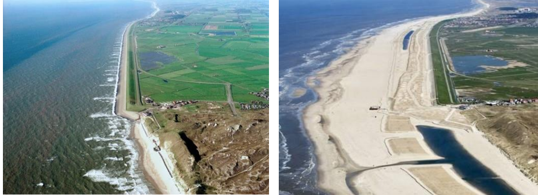
Figure 2. Left figure: Situation prior to construction in 2014, taken from Camperduin (South). The old sea dike is depicted as the primary flood defense system. Right figure: Situation immediately post construction in 2015. The Hondsbossche Dunes is constructed seawards of the old sea dike and has increased locally the coastal safety. Adapted from (Oudesluis, 2012).
