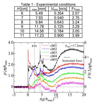
Figure 1 - Time variation of non-dimensional pressure and horizontal force acting on the vertical wall in the case of *H*=9cm
