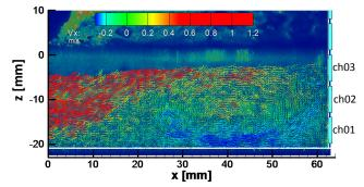
Figure 5 - Internal velocity field in front of the rectangular model at the time of "PIV2" indicated in Figure 3
