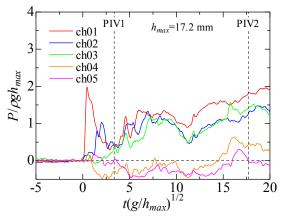
Figure 3 - Time variation of non-dimensional pressure acting on the rectangular model in the case of H=9 cm
