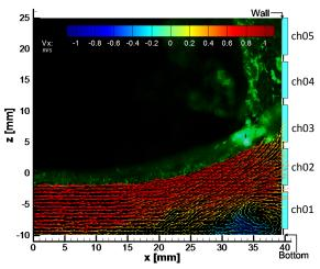
Figure 2 - Internal velocity field in front of the vertical wall at the time of "PIV" indicated in Figure 1
