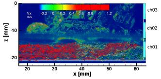
Figure 4 - Internal velocity field in front of the rectangular model at the time of "PIV1" indicated in Figure 3
