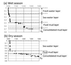
Figure 2 - Observed vertical profiles of bulk density at Stn B1 in (a) wet season and (b) dry season.
