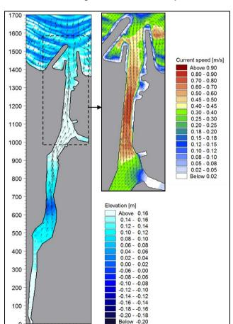
Figure 8. Phase Resolving Wave Model Snapshot (left) and Associated Currents (right)
