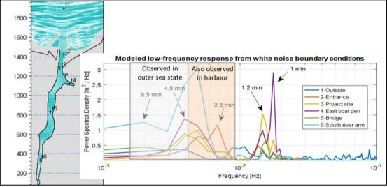
Figure 7. Results of White Noise Simulation with BW Model, Showing Natural Oscillation Frequencies
