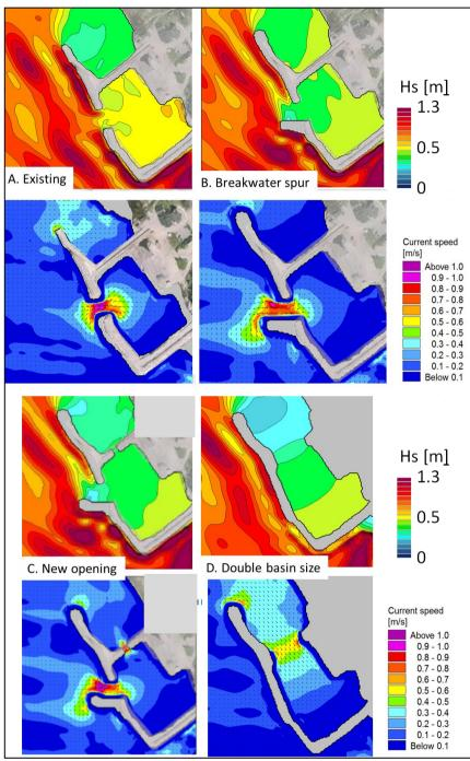
Figure 6. Sample modeled Hs (including swells + resonance) and resonance currents (right) at Harbour 1 for various basin reconfiguration options
