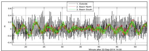
Figure 3. Sample surface elevation time-series from Harbour 1 wave gauges (1 outside, 2 inside the basin)
