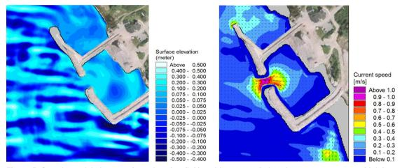
Figure 5. Sample modeled sea surface elevation (left) and long-wave induced resonance currents (right) at Harbour 1
