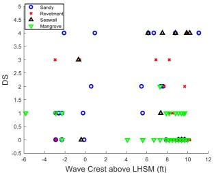
Figure 2: Structural damage state plotted against the elevation of wave crest above the structure's lowest horizontal structural member, classified by shoreline type: sandy beach (blue circles), revetment (red exes), seawall (black upward triangles), and mangrove (green downward triangles).
