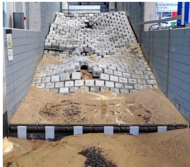
Figure 17. Dike after overflow event on previously damaged revetment (five stones had been pulled out).
