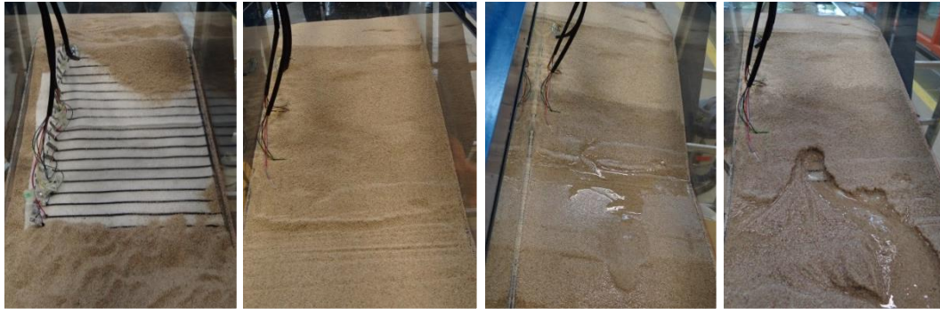
Figure 12. Placement of smart geotextile on the landward slope of small-scale dike model and development of water emersion and sand erosion at landward slope.
