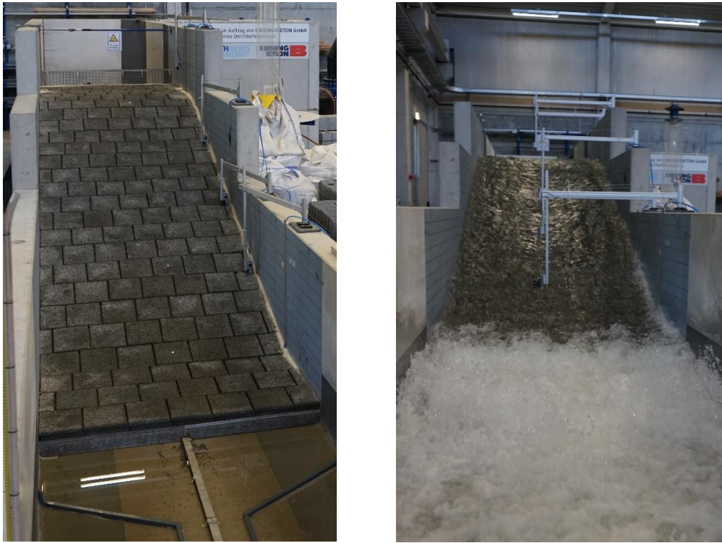
Figure 11. Large-scale dike model (left: overview; right: during overflow event, instrumentation in use).
