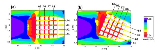
Fig. 3. The velocity distribution for the (a) aligned city buildings and the (b) skewed city buildings relative to the incoming flow at T=5.0 s
