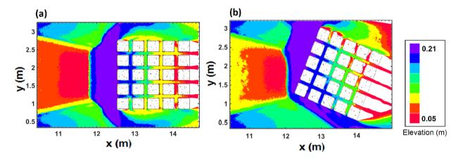
Fig. 2: The water elevation distribution at T=5 s and for buildings aligned at a (a) zero and (b) 22.5° angle relative to the approach flow direction.
