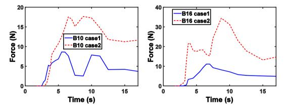
Fig. 4. The net impact force magnitude at building 10 and 16 indicated in figure 1.
