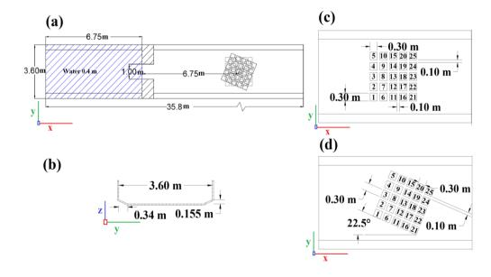
Fig. 1. The model setup: (a) the schematic view for the model setup, (b) the channel cross section, (c) buildings aligned at a zero (Case 1) and (d) buildings aligned at 22.5° angle relative to the approach flow direction (Case 2)
