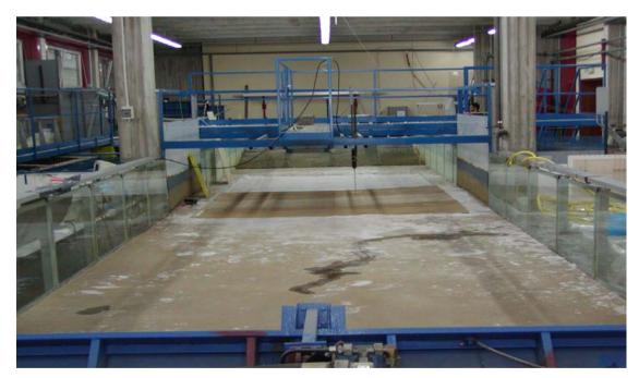
Figure 1 Picture of the experimental set up with the PVC rippled bed .
