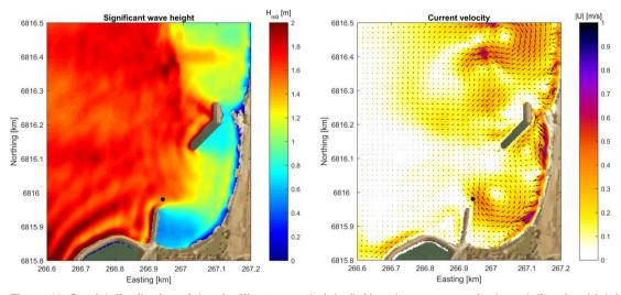
Figure 12: Spatial distribution of the significant wave height (left) and current magnitude and direction (right) for the option with <u>a 100 m breakwater extension</u>. Offshore condition:  $H_{m0} = 1.5$  m,  $T_p = 12$  s and  $\theta_p = 270^{\circ}$ N.
