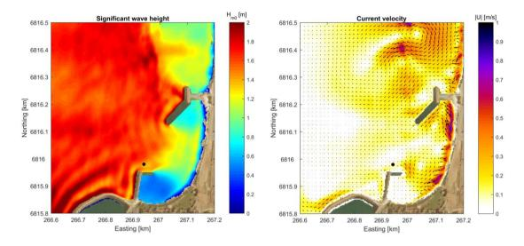
Figure 13: Spatial distribution of the significant wave height (left) and current magnitude and direction (right) for the <u>proposed</u> option consisting of a100 m breakwater extension, a connection to the shore and a 40 m spur attached to Batavia groyne. Offshore condition:  $H_{m0} = 1.5$  m,  $T_p = 12$  s and  $\theta_p = 270^{\circ}N$ .
