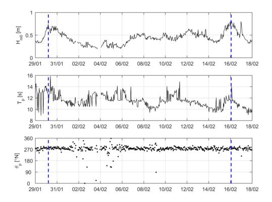
Figure 3: Part of the measured wave time series during Deployment 2. Vertical dashed blue lines indicate the events that have been used for validation of the SWASH model.
