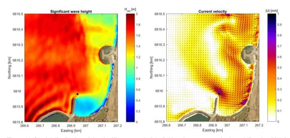
Figure 11: Spatial distribution of the significant wave height (left) and current magnitude and direction (right) for the <u>artificial headland</u> option. Offshore condition:  $H_{m0} = 1.5$  m,  $T_p = 12$  s and  $\theta_p = 270^{\circ}$ N.
