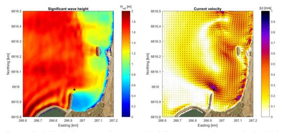
Figure 10: Spatial distribution of the significant wave height (left) and current magnitude and direction (right) for the <u>present</u> situation. Offshore condition:  $H_{m0} = 1.5 \text{ m}$ ,  $T_p = 12 \text{ s}$  and  $\theta_p = 270^{\circ}\text{N}$ .
