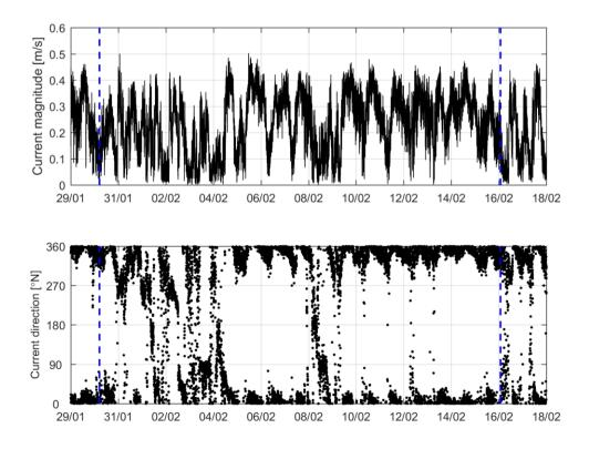
Figure 4: Part of the measured current time series (currents at z=0.4h) during Deployment 2. Vertical dashed blue lines indicate the events that have been used for validation of the SWASH model.
