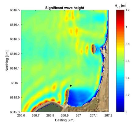
Figure 6: Spatial distribution of the significant wave height of wave Event 1.
