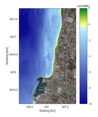
Figure 5: Outline and bathymetry of the Beresford Foreshore SWASH model
