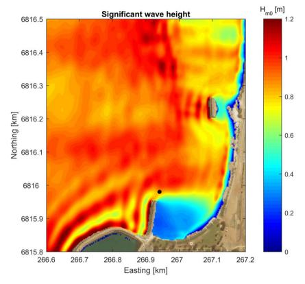
Figure 8: Spatial distribution of the significant wave height of wave Event 2.
