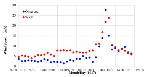
Figure 12. Results of wind speed of the simulation and observation at the Central Meteorological Observatory.
