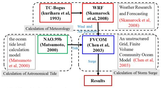
Figure 4. Model flow of the Coupled meteorology-ocean-tide model
