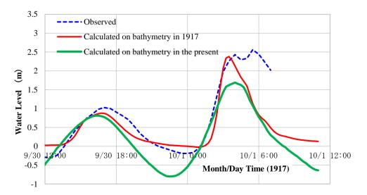
Figure 13. Comparison of water level height at Komatsugawa.
