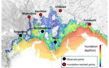
Figure 14. Inundation area on past bathymetry of 1917
