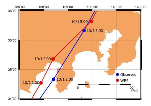
Figure 10. Results of calculated typhoon track compared with the observation presented by The Central Meteorological Observatory.
