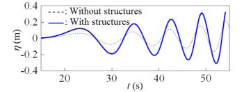
Figure 8. Numerical calculation results of water surface displacements at Point D shown in Fig. 7, in the cases with and without the wave concentration structures and Reef A.
