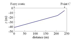
Figure 6. Distribution of still water depth along the shortest line between the ferry route and Point C shown in Fig. 5.
