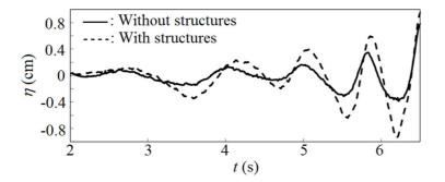
(b) Water surface displacements at the location of Wave gauge 2
