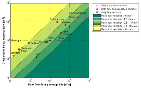
Figure 2: Relation between cross-section and maximum flow during average tide
