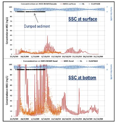
Figure 21: Comparison of suspended concentration at the surface and at the bottom
