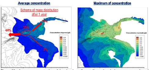
Figure 23: Average concentration of Lambarde sediment dispersion during one year and maximum concentration of Lambarde sediment dispersion during one year
