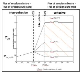
Figure 13: Variation of critical shear stress as a function of mass fraction of mud (Frvas) and relative concentrationof mud (Cv,rel), (B. Waeles, 2005)
