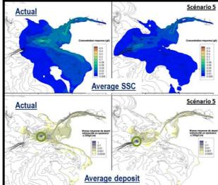
Figure 24: Exemple of comparison of dispersion between current situation and scenario 5
