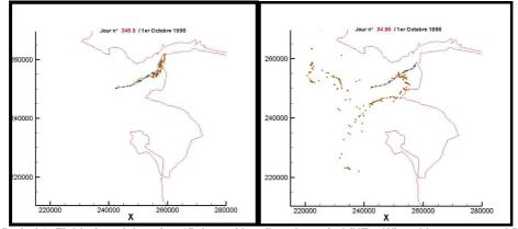
Figure 3 :Period 1: Field of particles after 15 days of low flow, low wind (NE ->W) and low waves and Period 3: Field of particles after 15 days of mean-> low flow, strong wind (W->NW), mean -> strong waves.
