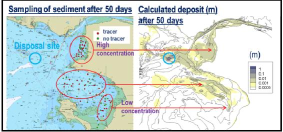
Figure 22: Comparison of tracer meausrement and deposit during 1 April-21 May
