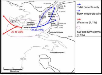
Figure 4: Preliminary study: establishing a first dispersion pattern
