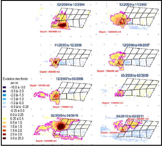
Figure 8: Evolution of Bathymetry
