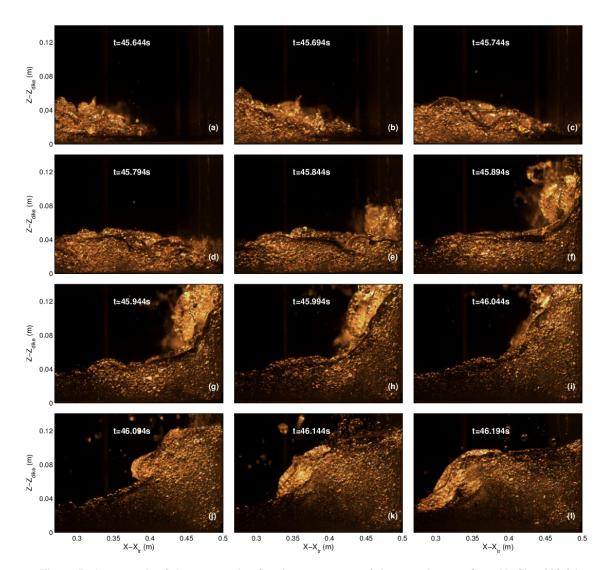
Figure 5: An example of the overtopping flow impact process of the second wave of test No.Sine-028-26. Note that  $x - x_{tr}$  and  $z - z_{dike}$  are the horizontal and vertical coordinate of dike crest. The wall is located at  $x - x_{tr} = 0.5$  m
