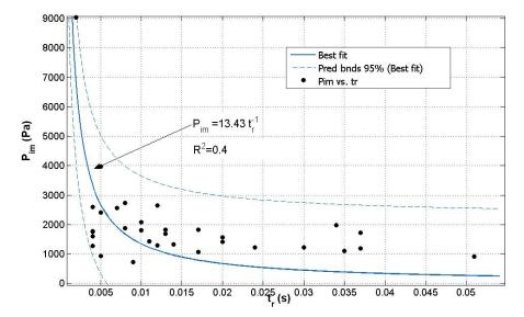
Figure 9: Re-plotting impact maximum pressure  $P_{im}$  and rising time  $t_r$  of  $P_1$  by forcing b=-1. Data points are from the 2nd and 3rd waves, as shown in Figure 8. Solid line is the best fit curve, and dashed lines are the 95% confidence interval.
