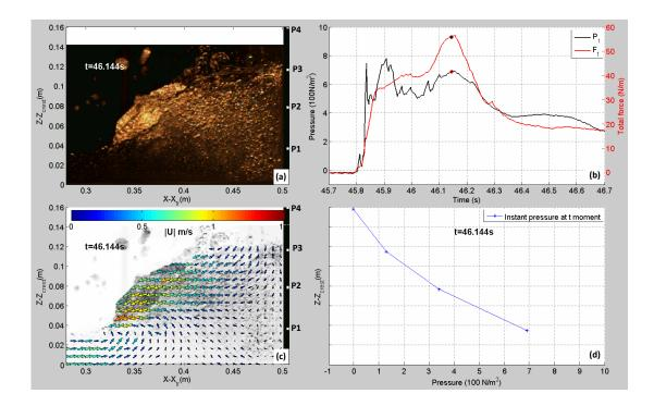
Figure 7: An example of measured flow field at the moment of the 2nd impact force peak occurrences. (a) raw high speed image at t=46.144 s; (b) impact time series of P1 (black) and total force obtained from load cell (red); (c) velocity filed at the t=46.144 s; and (d) instant measure pressure distribution at the same moment.
