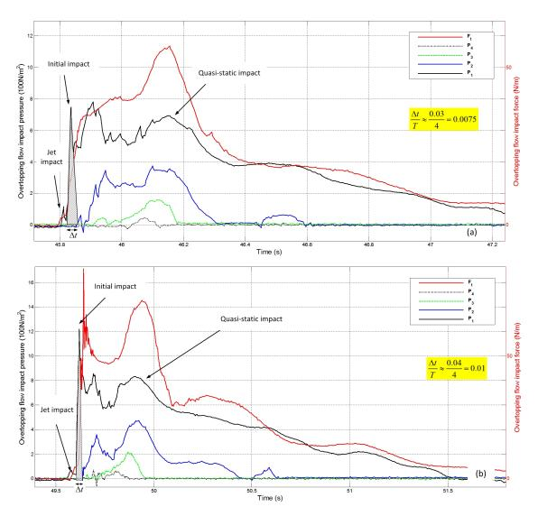
Figure 3: Example of the time series signals of total force from load cell and pressure sensors. (a) is from the second overtopping event shown in Figure and (b) is from the third event shown in Figure.  $\Delta t$  is the approximate impact duration and T is the incoming wave period
