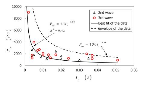
Figure 8: A relation of impact maximum pressure  $P_{im}$  and rising time  $t_r$  of  $P_1$ , triangle marker illustrates the data from the 2nd overtopping flow, whereas circles are the 3rd wave impact of each test.
