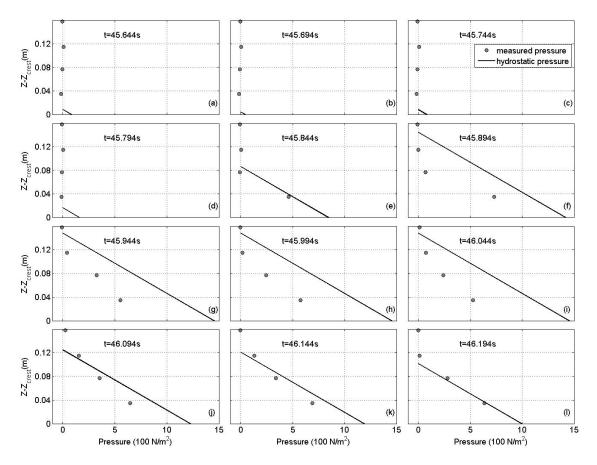
Figure 6: Instant measured pressure (gray marker) and computed hydrostatic pressure (=  $\rho g h_{max}$ ) (solid line),  $h_{max}$  is the highest water surface elevation at  $x_w$  extracted from raw image.
