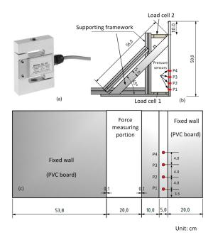
Figure 2: Wall model and force measuring system including (a) load cell (b) positioning of load cells and supported frameworks and (c) front view of wall model and locations of pressure sensors
