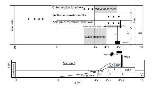
Figure 1: Wave flume in Flanders Hydraulic Research (Antwerp, Belgium). (a) is a top view of the flume, (b) is the respective section B to measure impact forces and velocity field.
