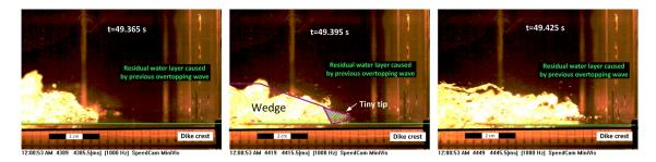
Figure 4: Snapshot of the third overtopping event of test No.Sine-028-26:  $H_0 = 0.2$  m,  $T_0 = 4$  s,  $h_0 = 1$  m, B = 0.5 m and  $\cot \beta = 3$ . The green line indicates the residual water level on dike crest. Note that the raw images have been adjusted by increasing the exposure value from 0 to 6.
