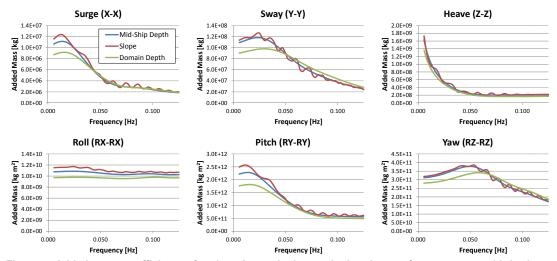
Figure 7. Added mass coefficients of tanker above sloping seabed and two reference cases with horizontal seabed
