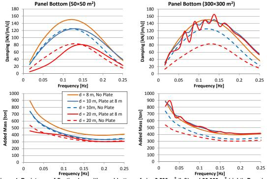
Figure 4. Resistance of floating box with panel bottom of size 2,500  $m^2$  (left) and 90,000  $m^2$  (right): Damping coefficients (top) and added mass coefficients (bottom) for heave (Z-Z)
