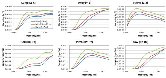
Figure 12. Damping coefficients of tanker above horizontal seabed (water depth 17 m, 23 m and 29 m)
