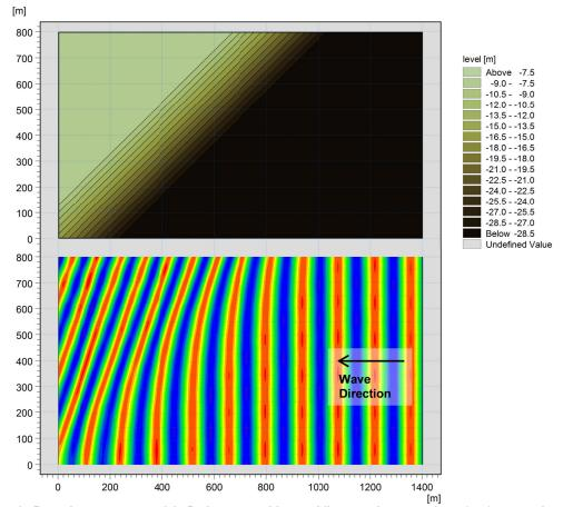
Figure 2. Boussinesq wave model: Bathymetry with an oblique underwater slope (top); monochromatic waves propagating across the slope (bottom)
