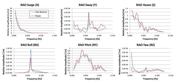
Figure 8. RAO's of tanker above sloping seabed in head on waves and two reference cases with horizontal seabed
