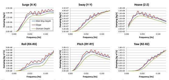
Figure 6. Damping coefficients of tanker above sloping seabed and two reference cases with horizontal seabed
