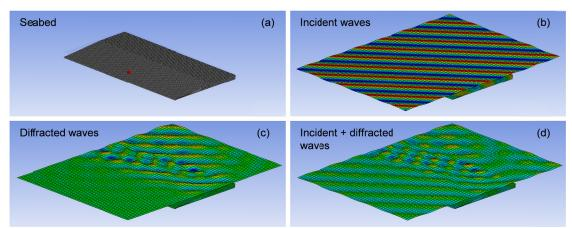
Figure 1. Waves over a sloping bottom in a panel model: (a) Panel model of the sloping seabed, (b) incoming waves, (c) diffracted waves and (d) superposition of incoming and diffracted waves
