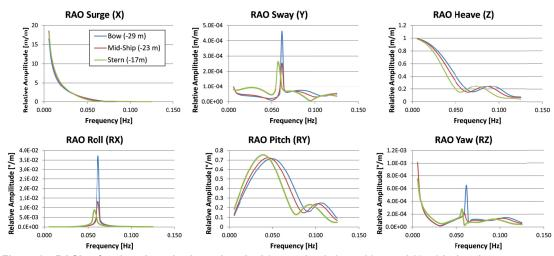
Figure 14. RAO's of tanker above horizontal seabed (water depth 17 m, 23 m and 29 m) in head on waves
