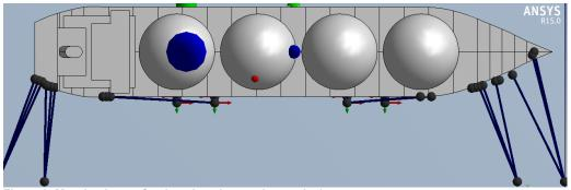
Figure 9. Mooring layout for time domain mooring analysis
