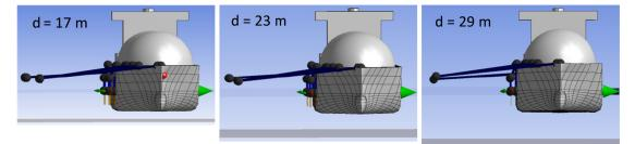
Figure 11. Tanker berth with horizontal seabed: Water depth 17 m (left), 23 m (centre) and 29 m (right)
