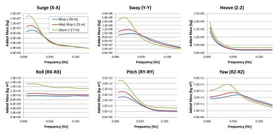
Figure 13. Added mass coefficients of tanker above horizontal seabed (water depth 17 m, 23 m and 29 m)
