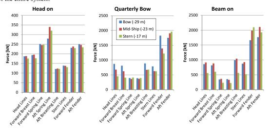
Figure 15. Line and fender forces above horizontal bottom (water depth 17 m, 23 m and 29 m)
