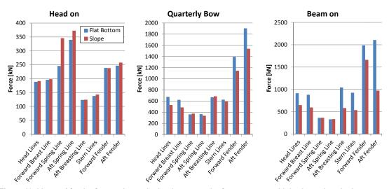
Figure 10. Line and fender forces above sloping bottom and reference cases with horizontal seabed
