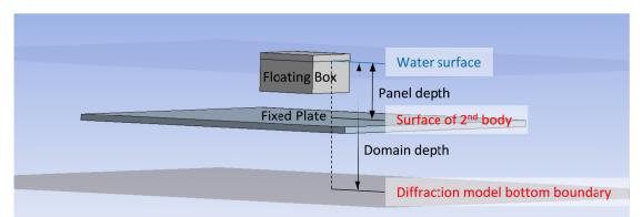
Figure 3. Panel model of floating box with domain depth of 20 m and panel seabed mode∥ (fixed plate) of size 50×50 m<sup>2</sup> with a panel depth of 8 m
