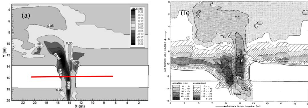
Fig 5 Comparison of the computed (a) and measured (b) bed level changes over 68 tides.
