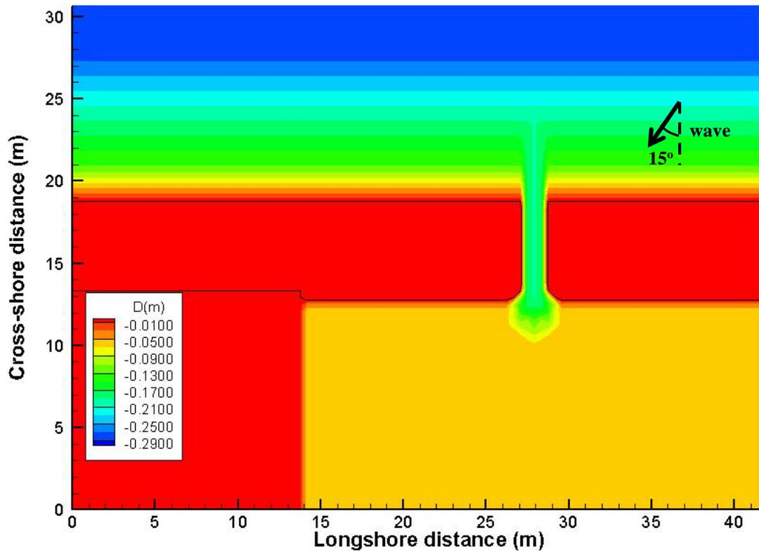
Fig 1 Layout of the computational domain and initial bathymetry.
