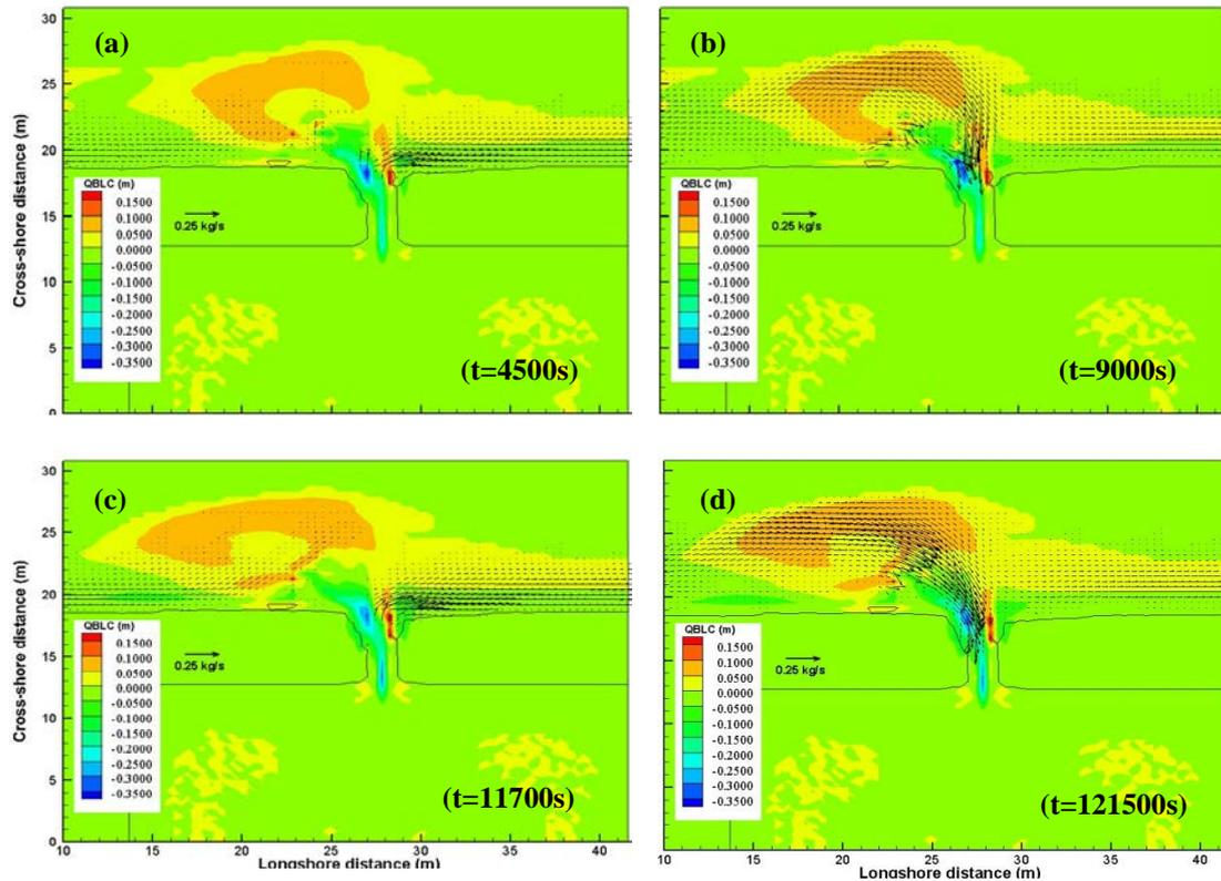
Fig 4 Distribution of computed sediment transport vector and bed level change at ebb (a), (c) and flood (b) (d).
