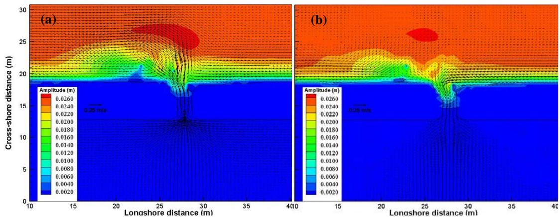
Fig 3 Computed flow velocity vectors and wave amplitudes at ebb (a) and flood (b).
