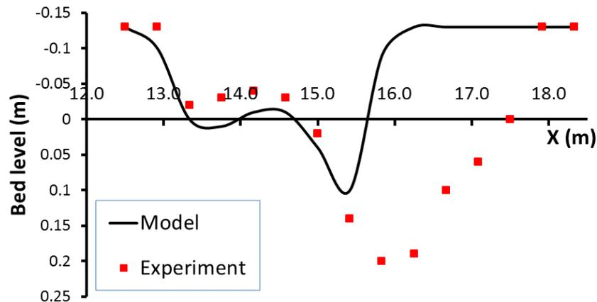
Fig 6 Comparison of computed and measured bed level along the section indicated in Fig 5(a) after 68 tidal cycles.
