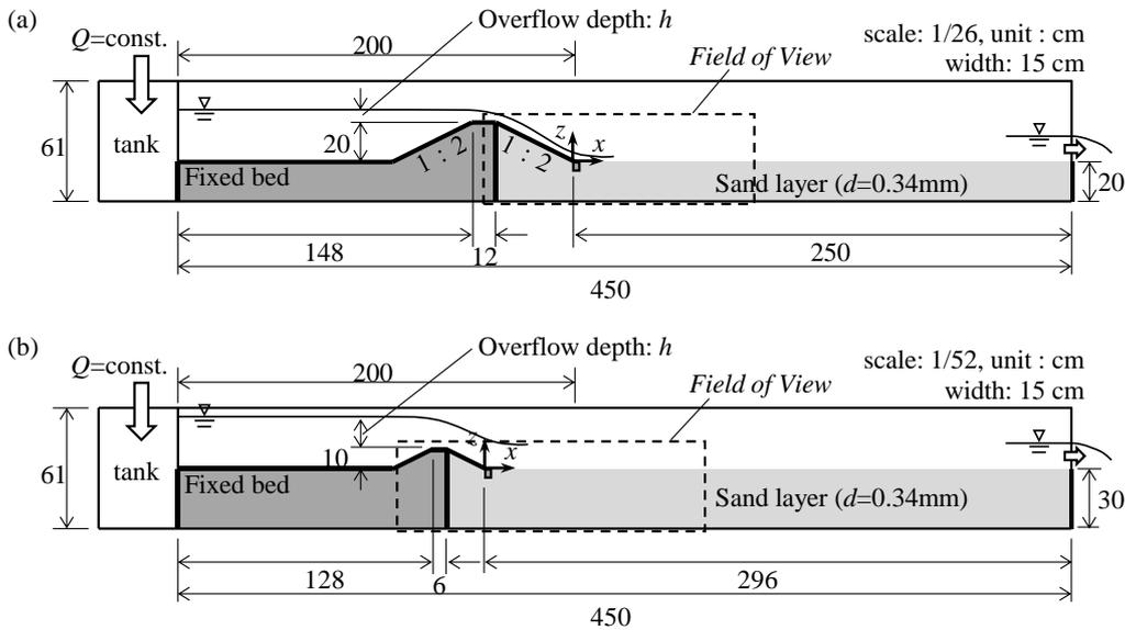
Figure 2. Experimental setup. (a) middle scale (1/26) model, (b) small scale (1/52) model.
