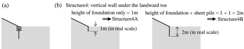
Figure 5. Schematic image of sheet-pile structure (a) and the model of the sheet-pile structure in this experiment (b).
