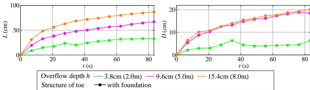
Figure 12. Temporal variations of the width and the depth of the scour holes with 1/52 scale model.
