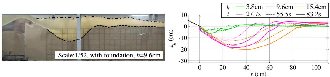
Figure 8. Results of the cases with higher overflow depth (case2-4-2-6).
