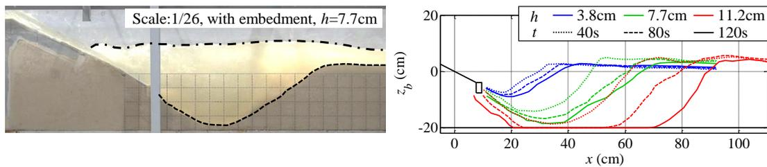
Figure 9. Results of the cases with embedment at the toe (case3-1~3-3).
