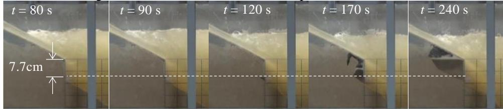
Figure 15. Results of the cases with the vertical wall under the toe (case4-1-4-2).
