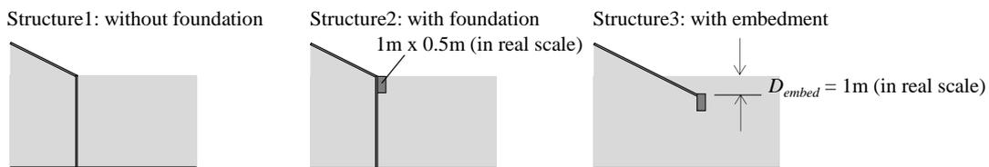
Figure 4. Structures of the landward toe of the coastal dike model.
