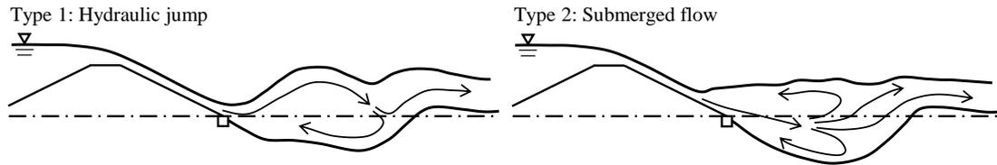
Figure 13. Two typical flow structures observed in the experiments.
