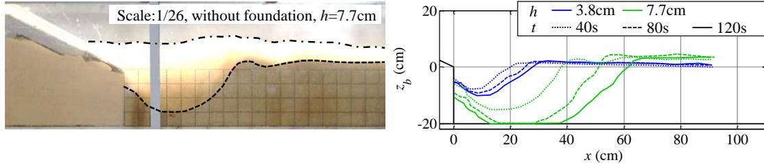
Figure 6. Results of the cases without foundation at the toe (case1-1-1-2).
