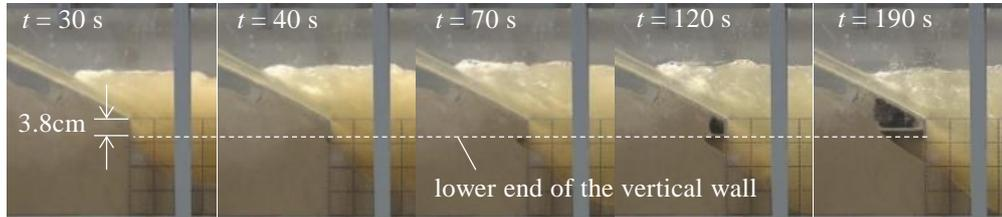
(b) case 4-2: height of the foundation and the sheet pile
