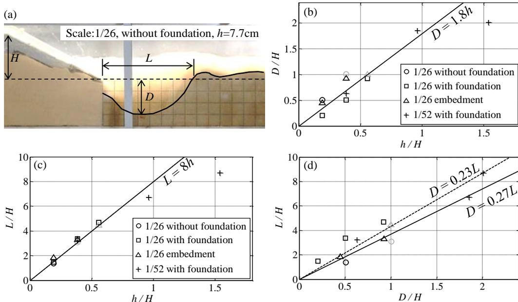
Figure 10. Relationship between overflow depths and sizes of scour holes. Definitions of depth  $D$  and width  $L$  of the scour hole are shown in (a). Dot line and Solid line in (d) show the empirical relationship based on the sizes of the scour holes observed after the 2011 tsunami by Tokida and Tanimoto (2012). Gray markers: results of the cases in which the scour holes reached the bottom of the channel.
