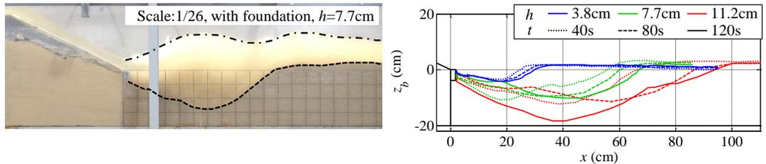
Figure 7. Results of the cases with foundation at the toe (case2-1-2-3).
