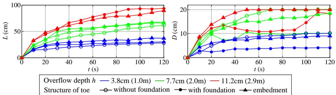
Figure 11. Temporal variations of the width and the depth of the scour holes with 1/26 scale model.
