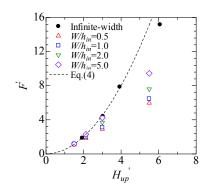
Figure 9. Relationship between the non-dimensional specific energy and the non-dimensional quasisteady force acting of the front face of a structure
