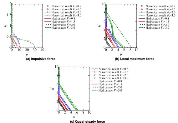
Figure 7. Pressure distribution acting on the front face of a structure in infinite-width structure case
