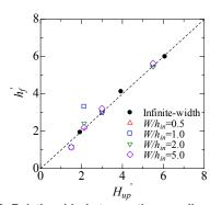
Figure 8. Relationship between the non-dimensional specific energy and the non-dimensional water level in the front of a structure
