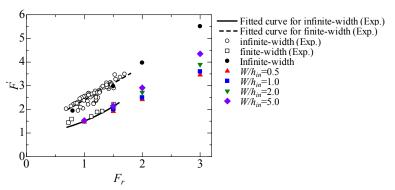
Figure 10. Comparison of the hydrodynamic force between measured in an early experimental study and predicted by our proposed method.
