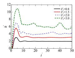
Figure 2. Time-history of the water level in front of a structure in infinite-width structure case
