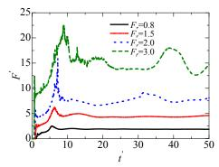
Figure 3. Time-history of the hydrodynamic force acting on the front face of a structure in infinite-width structure case
