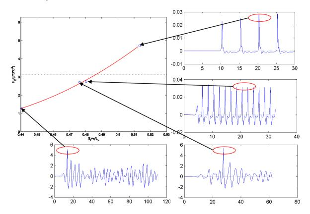
Figure 7 Relationship between slamming impact and wave front steepness
