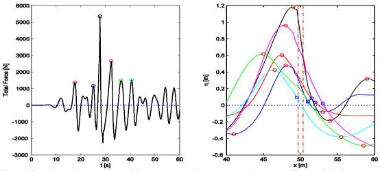
Figure 5 Snapshot of free surface at different time associated with the force peaks. The red dash line represents the pile.
