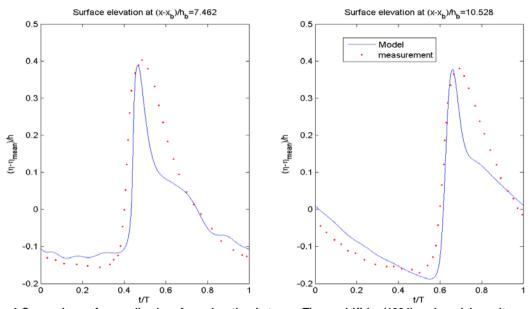
Figure 4 Comparison of normalised surface elevation between Ting and Kirby (1994) and model results.  $x_b$  and  $h_b$  are the coordinate and depth at the wave breaking point respectively,  $\eta$  is water surface elevation and h is water depth.
