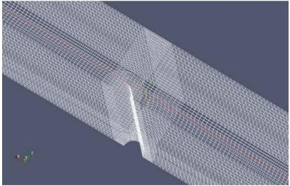
Figure 3 Example of computational mesh surrounding the monopile
