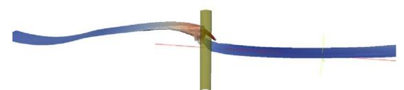
Figure 2 Snapshot of wave slamming on the monopile by OpenFOAM.
