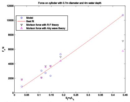
Figure 6 Relationship between total force on the pile and the wave front steepness for Case 1
