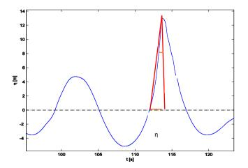
Figure 1 An example of surface elevation with a steep wave front and the definition of wave front steepness,  $S_{f}$ =tan( $\alpha)$ =\eta/L\_{\eta}.
