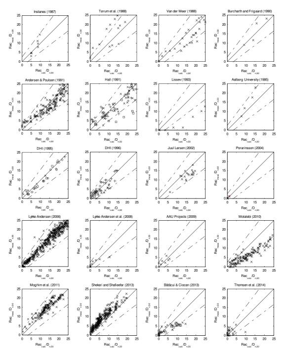
Figure 2. Evaluation of Lykke Andersen and Burcharth (2010) formula (Eq. 2) against the database. Red points are data outside validation area ( $h_s$ >h).
