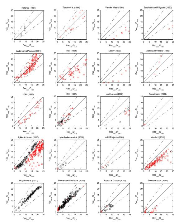
Figure 3. Evaluation of Moghim et al. (2011) formula (Eq. 3) against the database. Red points are data outside the validation area.
