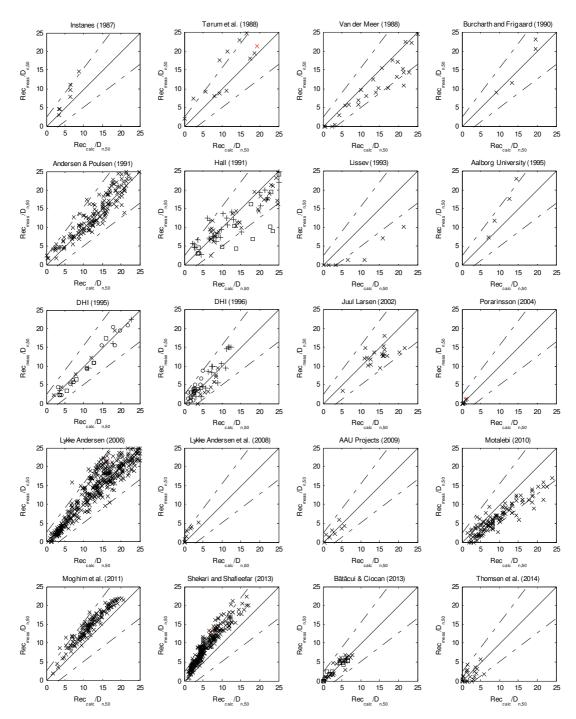
Figure 7. Evaluation of proposed updated Lykke Andersen formula (Eq. 8) against the database. Red points are data outside validation area ( $h_s$ >h).
