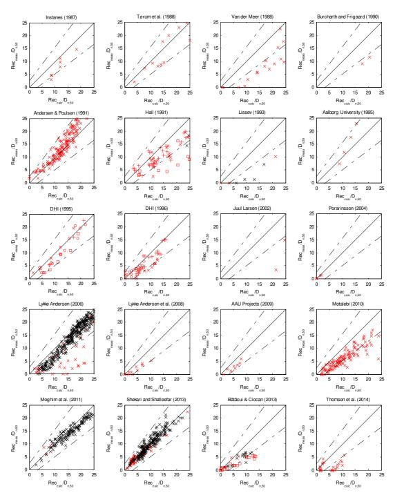
Figure 6. Evaluation of Moghim and Alizadeh (2014) formula (Eq. 6) against the database. Red points are data outside the validation area.
