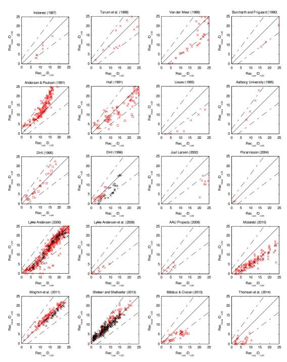
Figure 4. Evaluation of Shekari and Shafieefar (2013) formula (Eq. 4) against the database. Red points are data outside the validation area.
