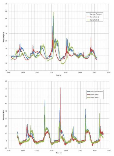
Figure 12: Example time series of spatially averaged uplift pressure from the F-P-F panels: a) the outer end of Pier I; b) the outer end of Pier III.
