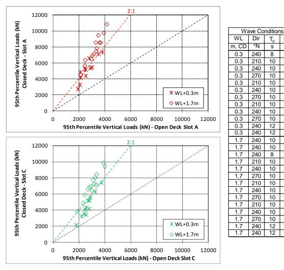
Figure 13: Reduction in peak uplift loads for the semi-open deck structure: a) force panel A; b) force panel C.
