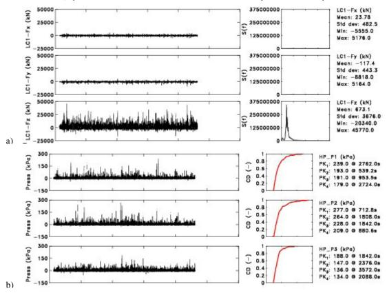
Figure 11: Typical graphical outputs from the GEDAP force and pressure analysis: a) time series and spectra for Fx, Fy, and Fz; b) time histories and cumulative distributions for three pressure sensors).
