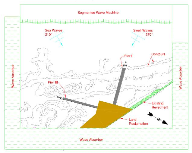
Figure 3: Physical model after bathymetry and port construction.
