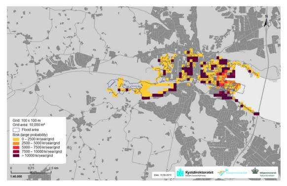
Figure 9. Flood risk mapping of Veijle, Denmark, for 2050 using flood risk assessment approaches from XtremRisK, units are in Danish crowns/year/grid cell.
