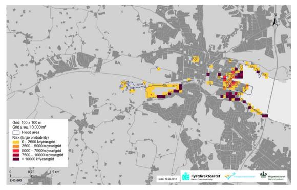
Figure 8. Flood risk mapping of Veijle, Denmark, for 2012 using flood risk assessment approaches from XtremRisK, units are in Danish crowns/year/grid cell.
