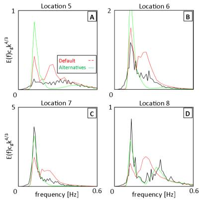
Figure 5. Observed and computed scaled variance density spectra for case 23:00 UTC of the Haringvliet data set at the four most shoreward locations. Spectra computed with the default source terms (LTA + BJ model) are shown in red (--) and the spectra computed with the alternative source terms ( $\beta - kd$  + mSPB) are shown in green (...). Note that the spectra are scaled so that a  $k^{-4/3}$  tail appears horizontal.
