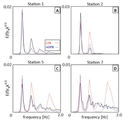
Figure 4. Observed and computed scaled variance density spectra for Case 31 of the Smith (2004) data set. Panels A to D show the evolution of the spectra in the surf zone from at the wave-maker (Location 1) to deep in the surf zone (Location 7). Spectra computed with the LTA are shown in red (--) and the spectra computed with the mSPB are shown in blue (..). Note that the spectra are scaled so that a  $k^{-4/3}$  tail appears horizontal.
