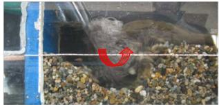
Figure 4 Scouring downstream of over flow
