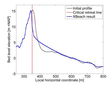
Figure 5: Approximate design point post-storm profile (XBeach).
