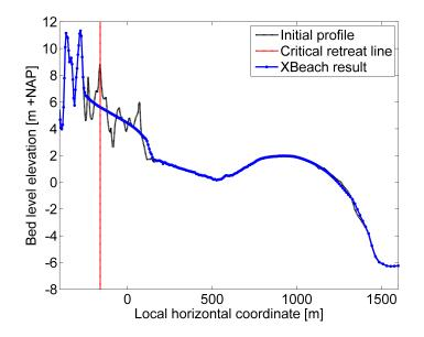
Figure 6: Approximate design point post-storm profile (XBeach).
