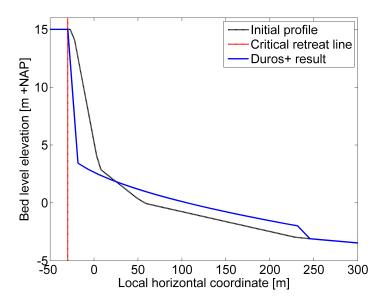
Figure 4: Design point post-storm profile (Duros+).
