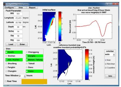
Fig.13 The user interface of local tsunami warning system for Taiwan's coastal regions.
