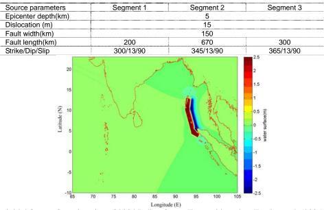
Table 1 The fault parameters for the 2004 Indian Ocean Tsunami.
