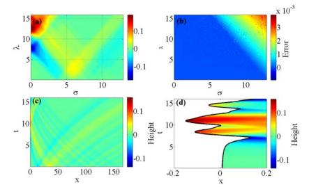
Fig.3 (a) The total mechanics energy  $\varphi(\sigma, \lambda)$  calculated by eq.(13), (b) the error distribution between eq.(10) and eq.(13), (c)the spatial and temporal variation of wave displacement in the physical domain(x, t) and (d) the variation of the wave displacement and the moving shoreline on the coastal region.
