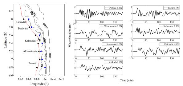
Fig.8 The distribution of offshore boundary points and their simulated time series with the sampling frequency 0.016 Hz on east coast of Sri-Lanka.
