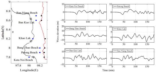
Fig.6 The distribution of offshore boundary points and their simulated time series with the sampling frequency 0.016 Hz on Phuket coast.
