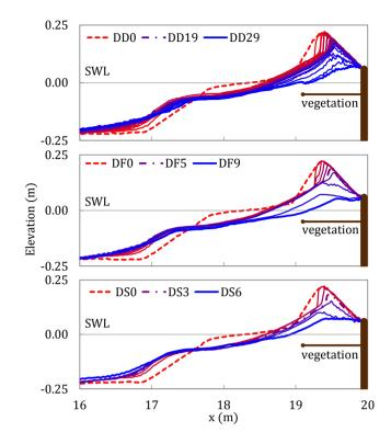
Figure 7. Measured dune profiles for DD, DF and DS tests.
