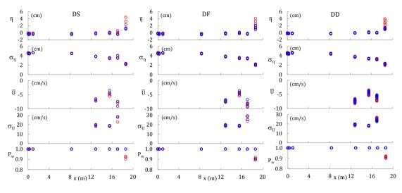
Figure 6. Measured mean and standard deviation of free surface elevation and cross-shore velocity together with wet probability P<sub>w</sub> for DS, DF and DD tests.
