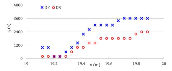
Figure 11. Measured landward progression of toppling time  $t_{t}$  in the middle of toppling run for DF and DS tests.
