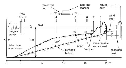
Figure 1. Schematic view of the experimental set-up including wave paddle, sandy beach profile on top of plywood slope, collection basin including sediment trap, water recirculation system, laser line scanner mounted to a motorized cart and location of the instruments measuring the hydrodynamics with a dune profile without wooden dowels.
