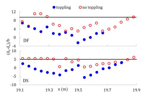
Figure 10. Burial depth ( $d_b$ - $d_e$ ) normalized by dowel diameter b before and after toppling run for DF and DS tests.
