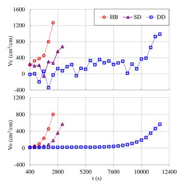
Figure 5. Temporal variations of cumulative sand volume change  $V_c$  and overwash volume  $V_o$  per unit width for HB, SD and DD tests.
