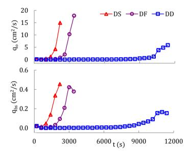
Figure 8. Temporal variations of wave overtopping rate  $q_0$  and sand overwash rate  $q_{bs}$  for DD, DF and DS tests.
