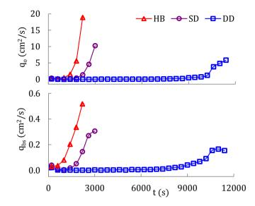
Figure 4. Temporal variations of wave overtopping rate  $q_{\text{o}}$  and sand overwash rate  $q_{\text{bs}}$  for HB, SD and DD tests.
