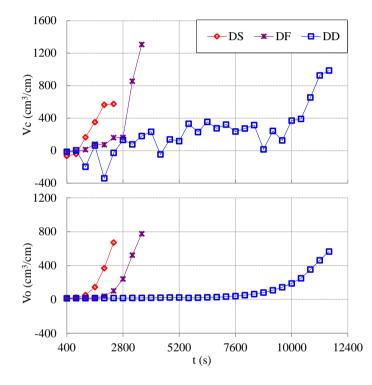
Figure 9. Temporal variations of cumulative sand volume change  $V_{\rm c}$  and overwash volume  $V_{\rm o}$  per unit width for DD, DF and DS tests.
