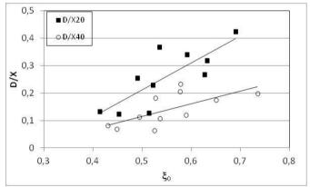
Figure 5 Dimensionless toe depositions against the surf parameter
