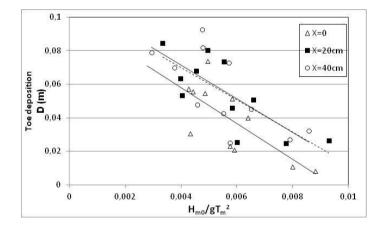
Figure 3 Variation of the toe deposition height with the wave steepness
