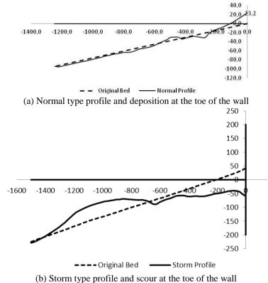
Figure 2 Development of the beach profile with the seawall in run-up region
