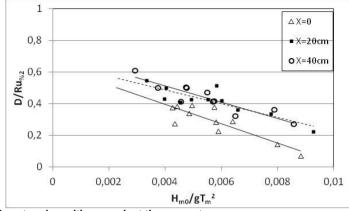
Figure 4 Dimensionless toe depositions against the wave steepness
