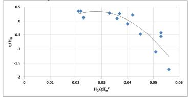
Figure 7 Dimensionless toe level variation against the wave steepness for 1:5 slope and for location X=20cm
