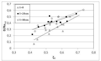
Figure 6 Dimensionless toe depositions against surf parameter
