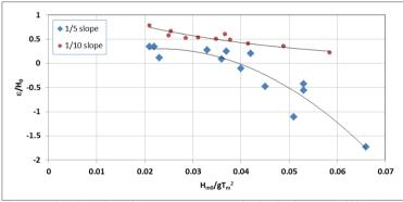
Figure 8 Dimensionless toe level against the wave steepness for both slopes and X=20cm
