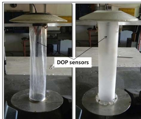
Figure 2. Tested devices: flexible (left) and rigid (right) types. DOP sensors are mounted into the tubes.
