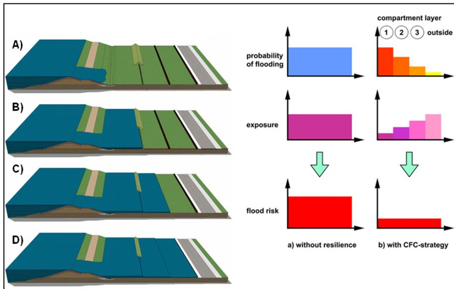
Figure 15. Principle of a system with flood compartment (left: flooding of the first, second and third compartment, right: risk reduction due the CFC-approach) (modified from Ujeyl et al. 2012).
