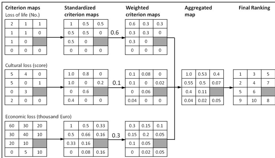
Figure 12. General integration procedure for different damage categories using the Simple Additive Weighting Method (SAW), (modified from Dassanayake et al. 2011).
