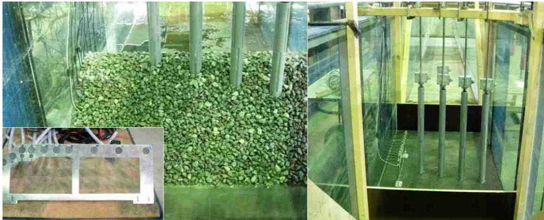
**Figure 8. Experimental setup in the flume. The mount with pressure sensors is shown on the left; the array with wave gauges is shown on the right; the centre image shows the complete structure.**
