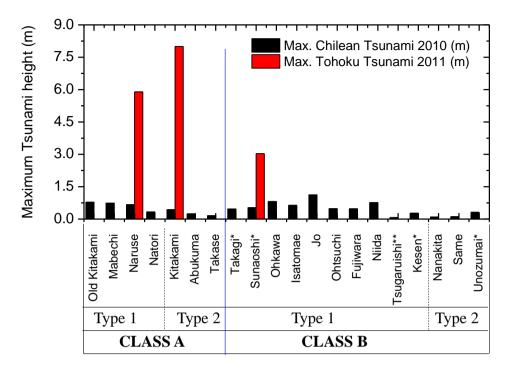
Figure 11. Comparison of maximum observed tsunami runup height at nearest river mouth stations for the 2010 Chilean Tsunami and 2011 Tohoku Tsunami
