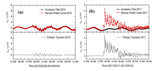
Figure 2. Measurement water level variation during the Chilean Tsunami 2010 and the Tohoku Tsunami 2011
