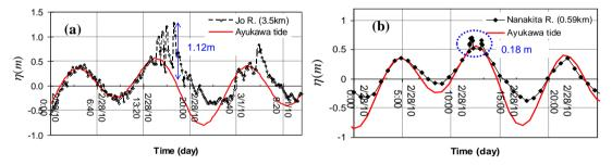
Figure 4. Tsunami responses to the Jo River (Type 1) and to the Nanakita River (Type 2)
