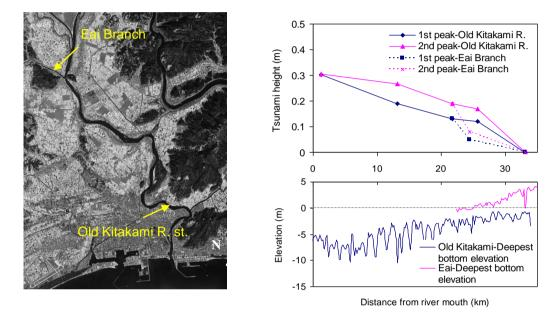
Figure 6. Old Kitakami River morphology and the variation of 1st and 2nd 2010 tsunami peaks along river
