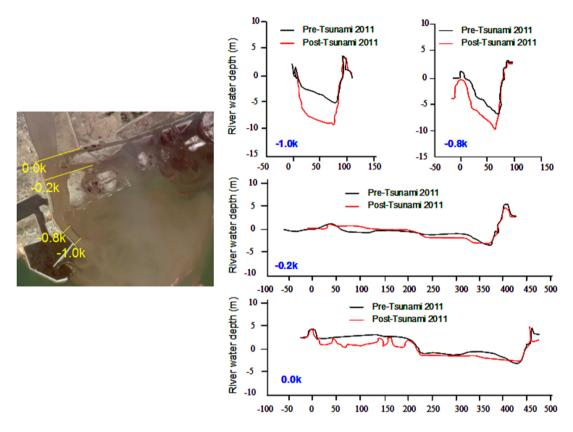
Figure 10. Deeping of river bed elevation at the Natori River
