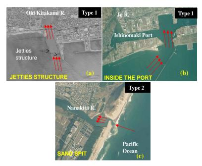
Figure 3. Classification of Type 1 River (Full-width energy intrusion) and Type 2 River (Divergent wave energy intrusion)
