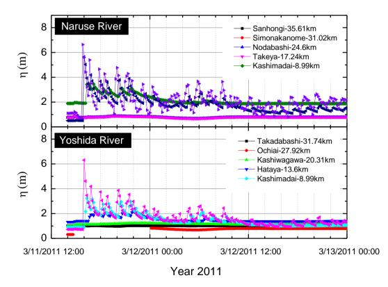
Figure 9. The 2011 Tsunami variations along the Nasure and Yoshida Rivers
