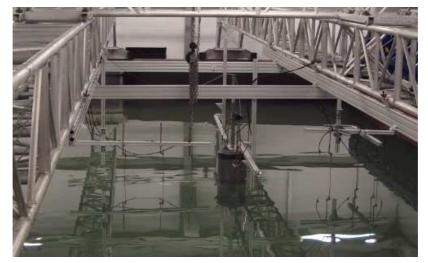
Figure 3. The developed generic point absorber WEC during experiments in the wave basin of Queen's University Belfast, Northern Ireland, UK.
