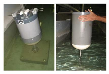
Figure 2. The developed generic point absorber WEC during experiments in the wave flume of Ghent University, Belgium.
