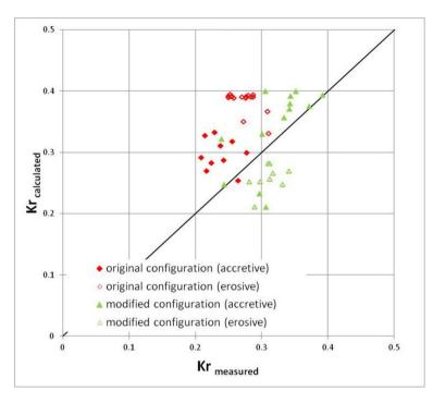
Figure 9. Comparison between the reflection coefficients measured and calculated by using the analytical model of Gonzalez et al. (1999).
