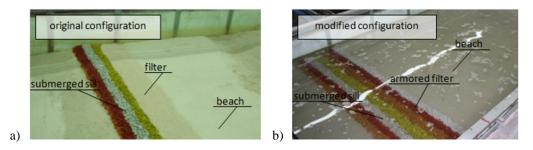
Figure 6. Investigated configurations of the perched beach nourishment: a) original configuration; b) modified configuration (where the filter has been covered with a layer of elements similar to those of the submerged sill).
