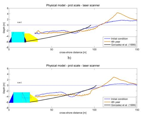
Figure 10. Comparison between the beach profiles measured and calculated by using the analytical model of Gonzalez et al. (1999) at prototype scale. The initial beach profile in blue is reported as a reference condition. The blue structure is the rubble mound sill, the yellow area represents the filter, the cyan region is the equivalent impermeable rectangular barrier considered in the application of the analytical model. a) original configuration; b) modified configuration.
