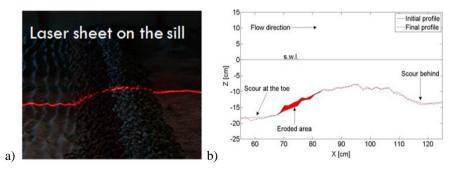
Figure 5. 2D computer vision system for recovery the damage to the submerged barrier and the scour depth close to it. a) formation of the image; b) interpretation of the image to measure the eroded area and the scour depth in front and behind the sill.
