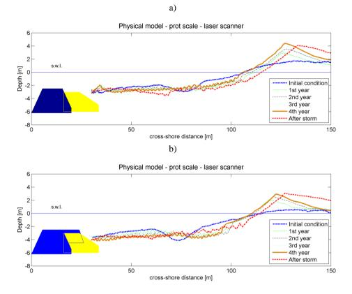
Figure 7. Evolution of the beach profile measured at the end of several series of accretive waves (1<sup>st</sup> year, 2<sup>nd</sup> year, 3<sup>rd</sup> year and 4<sup>th</sup> year, each year is made up by about 12500 waves) followed by a series of erosive wave (small storm having about 2 years return period). a) original configuration; b) modified configuration. Measurements are reported at prototype scale.
