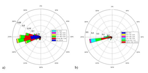
Figure 3. Directional distribution of significant wave height at the site of interest. a) Frequency of significant wave height in deep waters. b) Frequency of significant wave height at closure depth (h=7.2 m).
