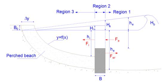
Figure 1.Sketch of the problem and definition of the variables of the analytical model (adapted from Gonzalez et al. 1999).
