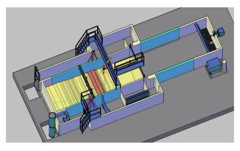
Figure 4. Experimental wave tank and location of the physical model of the perched beach nourishment (the barrier is in red), and of the measurement instruments.
