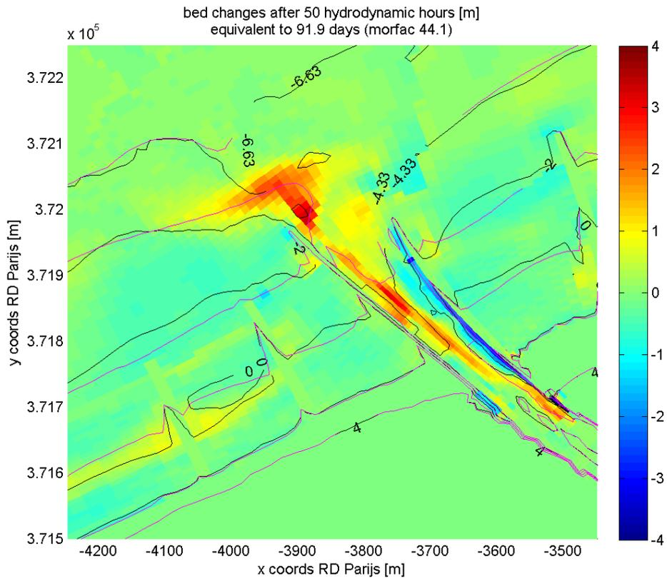
Figure 9 : Modelled erosion-sedimentation pattern after three months.
