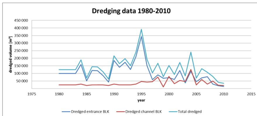
Figure 2 : Dredged volumes in the entrance channel of Blankenberge (Houthuys, 2012), seaward of the groynes (dark blue), between the groynes (red) and total dredged volumes (light blue).
