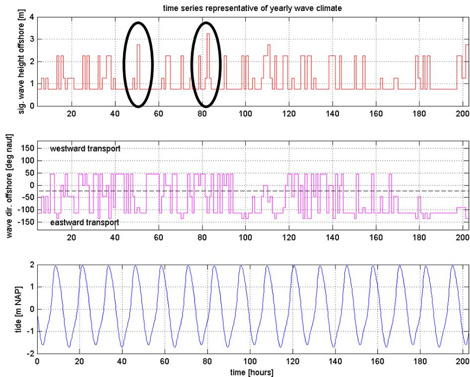
**Figure 8 :** Time series of wave conditions used at the offshore boundary of the Delft3D model in the constant morfac approach, with significant wave height (red), wave direction (magenta) and water level (blue). Storm events mentioned in Figure 12 are circled in black.
