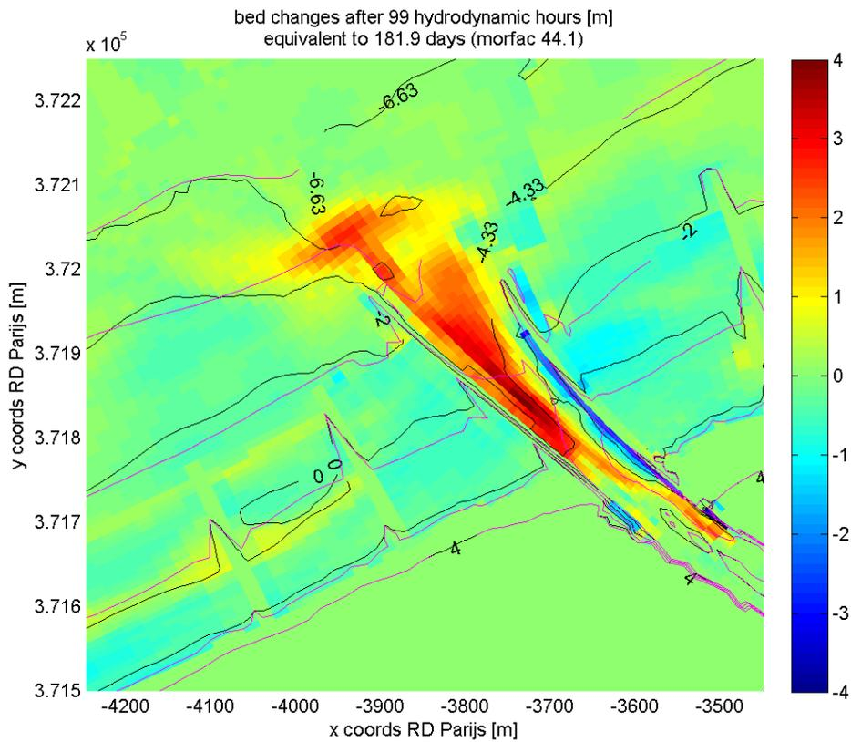
Figure 10 : Modelled erosion-sedimentation pattern after six months.
