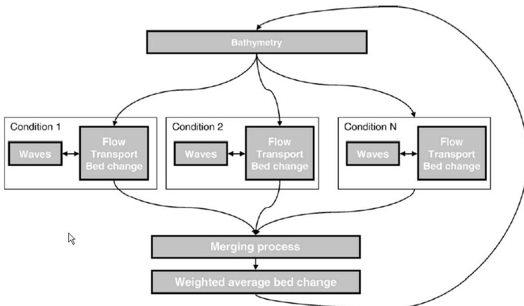
**Figure 7 : Schematisation of the MorMerge process for morphological modelling with a reduced wave climate. Figure from Lesser (2009).**
