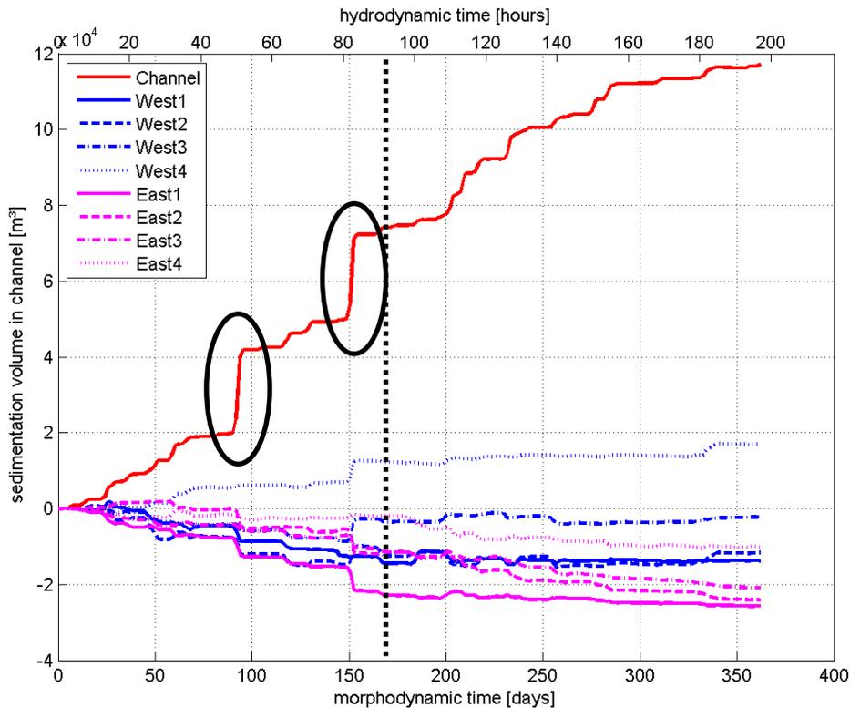
**Figure 12 : Cumulative erosion-sedimentation in the entrance channel of Blankenberge and in each groyne section on both sides of the channel (numbered from 1 to 4: closest to furthest from the channel). Black circles correspond to storm events leading to strong sedimentation in the channel.**
