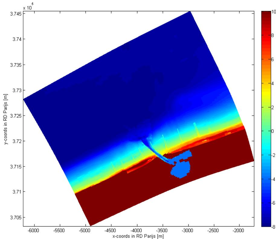
**Figure 4 : Bathymetry of the Blankenberge model, in RD Parijs coordinates and relative to NAP level (equivalent to MSL).**
