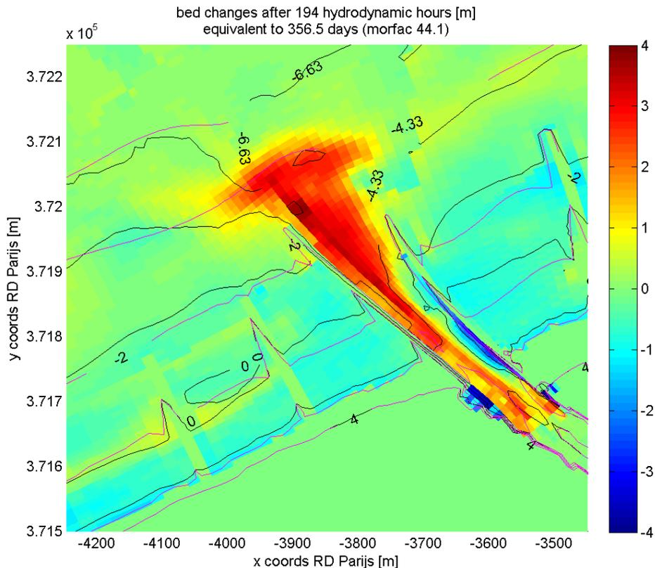
**Figure 11 : Modelled erosion-sedimentation pattern after around one year.**
