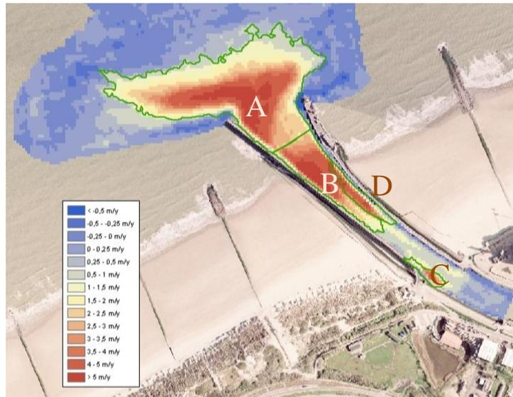
Figure 1: Estimated yearly sedimentation in the entrance channel, scale from -0.5 m/year (blue) to +5 m/year (red) (reproduced from Teurlinx et al., 2009).
