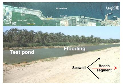
Figure 10: View of wave flooding over the beach segment after the December 2010 storm
