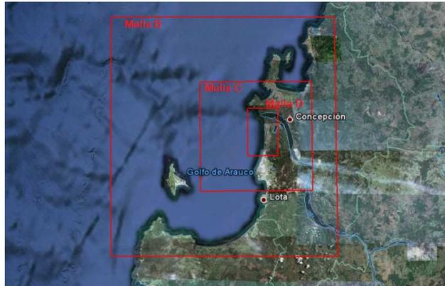
Figure 2. Grids B, C and D with 27", 9" and 3" spatial resolution, respectively, which were used in the numerical simulations
