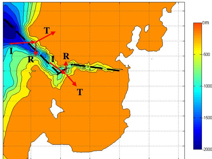
Figure 8. Bathymetry of the Biobio canyon with contour lines every 200m. The dashed lines represents the main segments of the canyon and the red arrows shows incident (I), reflected (R) and transmitted (T) tsunami waves.
