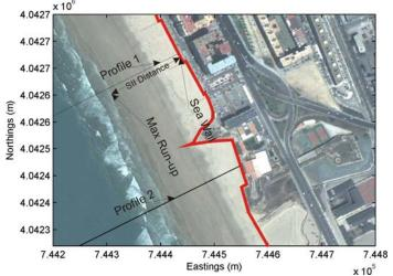
Figure 6. Schematic representation of the SII used at the urban beach of the city of Cadiz
