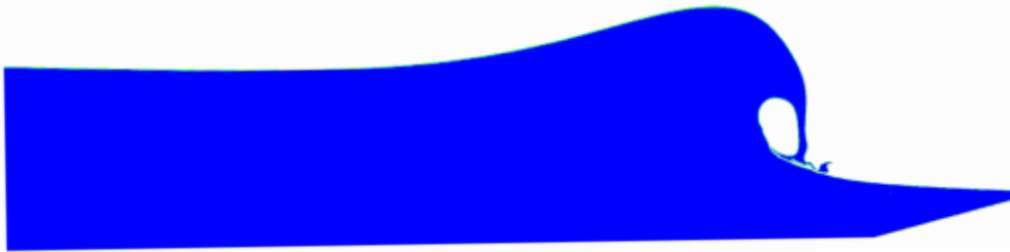
Figure 4. Type 1 solitary wave breaking. VOF-PLIC method. C \geq 0.5 . Slices taken in the middle of the 3D numerical domain.
