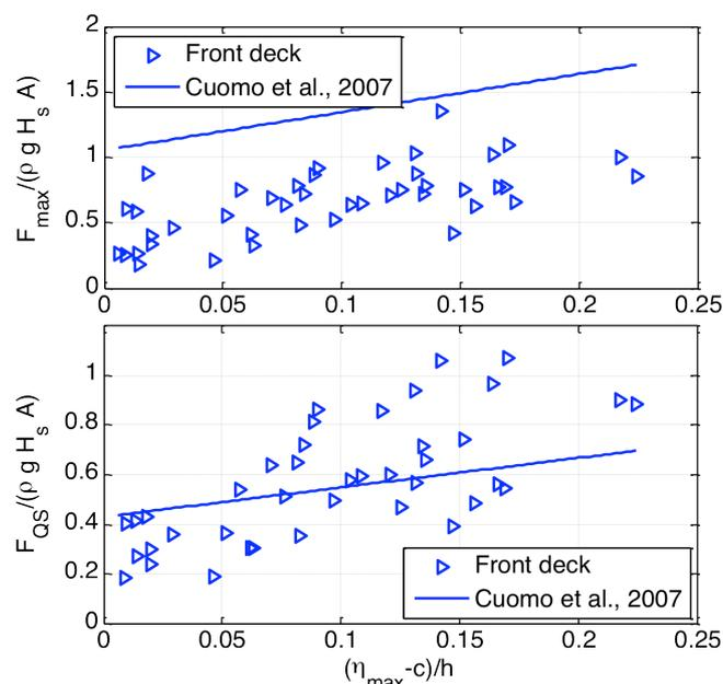
Figure 14. Maximum (top) and quasi-static (bottom) horizontal forces under irregular waves: comparison with small-scale results (Cuomo et al. 2007).
