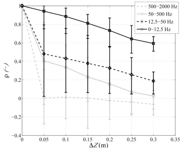
Figure 6. Measured force correlations on deck front versus separation  $\Delta Z$  for different frequency bands (from Lamberti et al. 2011).
