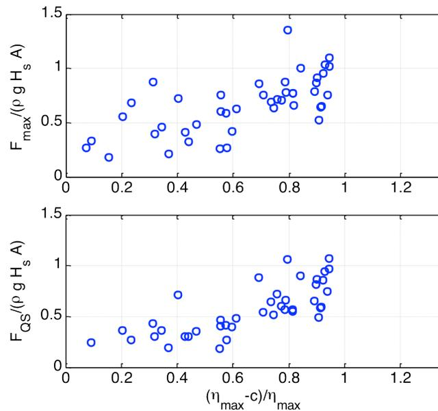
Figure 12. Forces on front deck under irregular waves: quasi-static (bottom) and maximum (top) values.
