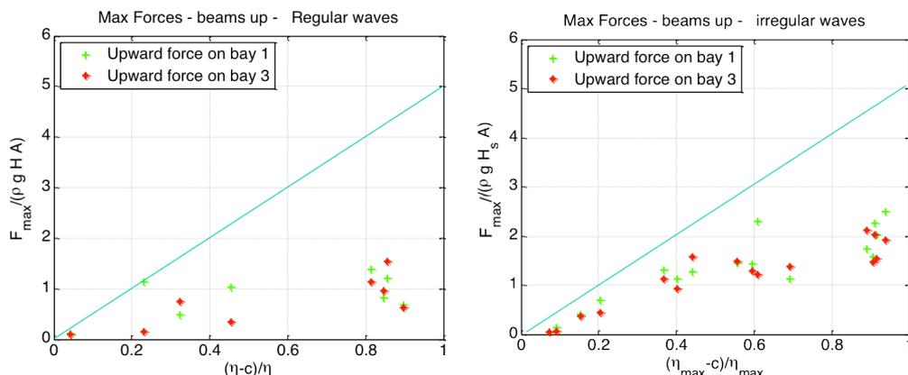
Figure 10. Beams up: maximum forces on bay 1 and 3 under regular (left) and irregular (right) waves.
