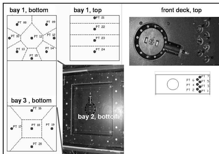
Figure 4 Position of pressure transducers on deck soffit of bay 1, bay 3, on topside of bay 1, on the front side, with (---) influence area of each transducer used for total force calculation.
