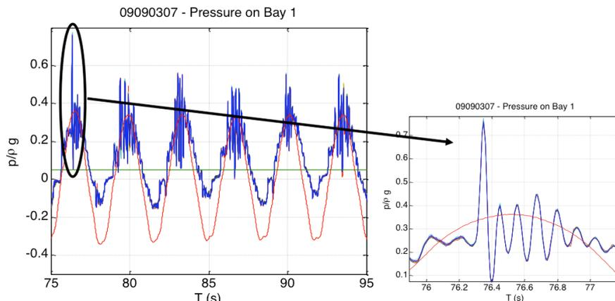
Figure 8. Regular wave test: pressure signal in time on bay 1.
