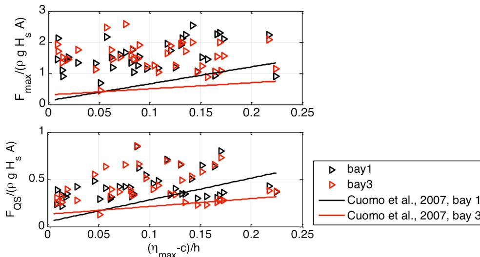
Figure 13. Maximum (top) and quasi-static (bottom) upward forces under irregular waves: comparison with small-scale results (Cuomo et al. 2007) for beams up configuration.
