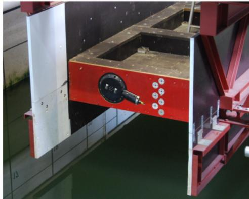
Figure 3. Front view of the model deck and of the overbearing retaining structure. The positions of the PAU and some pressure transducers on the deck front are also shown.
