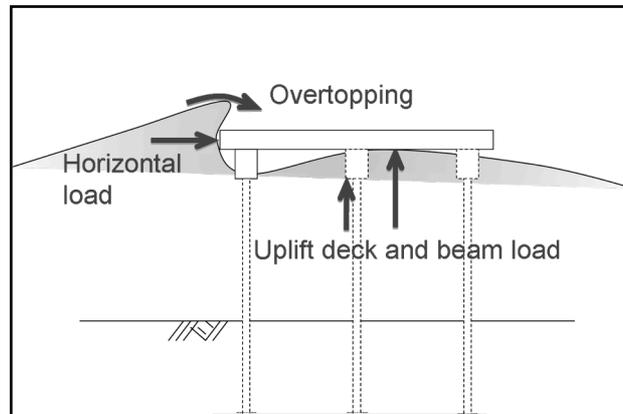
Figure 2. Sketch of wave-induced forces on a typical jetty (from Lamberti et al. 2011).
