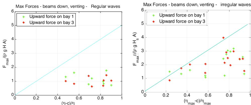
Figure 11. Maximum forces on the bay 1 and 3: configuration beams down vents: regular (left) and irregular (right) waves.
