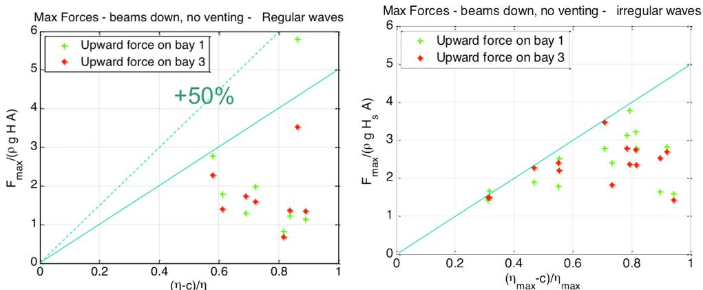
Figure 9. Beams down: maximum forces on bay 1 and 3 under regular (left) and irregular (right) waves.
