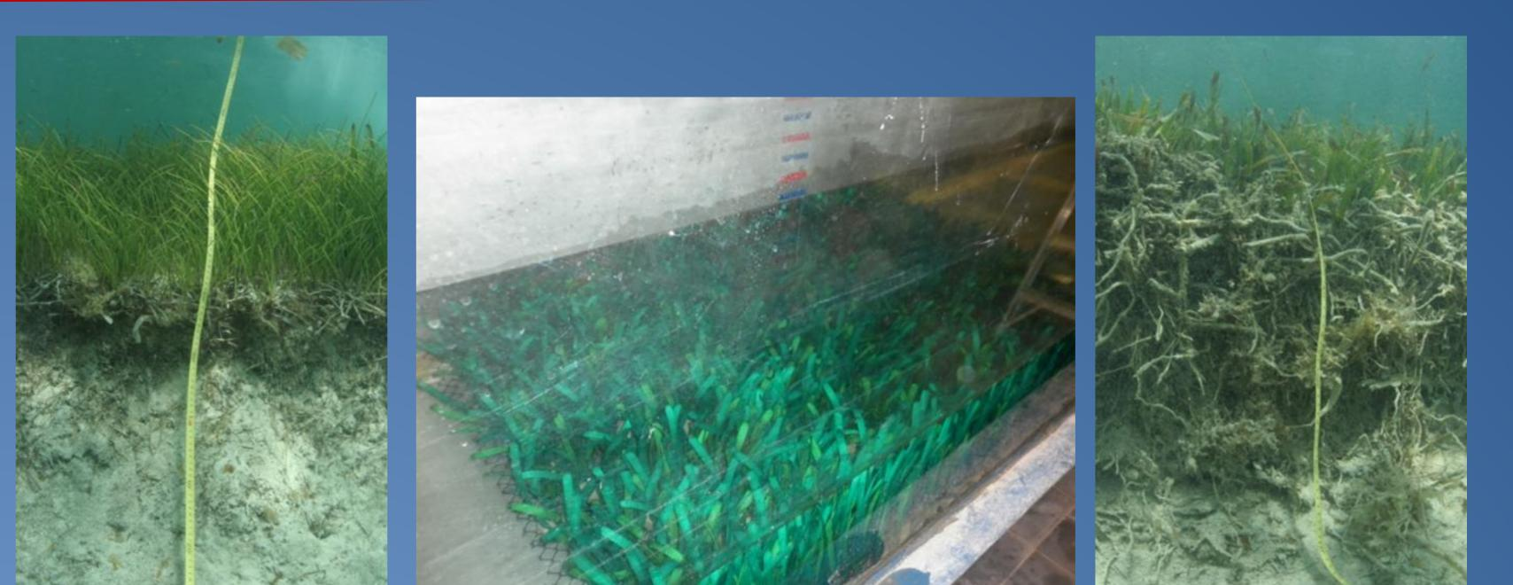
The work described in this poster aims to determine the performance of a patch of seagrass in terms of the energy loss of the waves travelling through it; to do so several wave conditions, water depths and different vegetation densities were tested in laboratory experiments using a synthetic hand-made seagrass patch.
