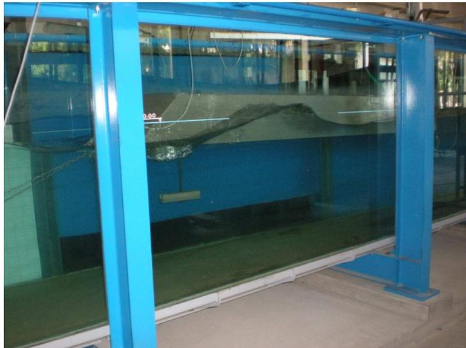
Figure 8. The SeaBreath tested in the wave flume at Padova University.
