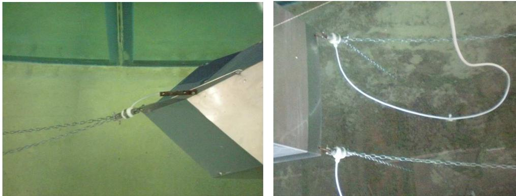
Figure 12. Load cells mounded along the front and rear chains.
