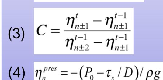
The phase speed *C* is estimated by Eq. (3) with the variables in the interior grids.
