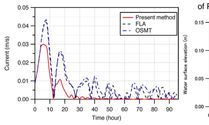
Fig. 3. Comparisons of calculated currents for different OBCs at the grid point B in the case of PIC.
