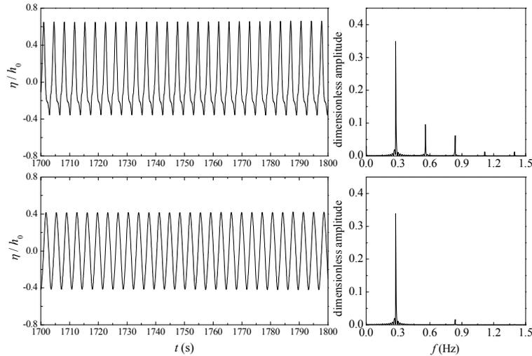
Fig. 7 Free surface elevation and amplitude spectrum corresponding to transverse oscillations estimated by the difference in time history recorded by probes S1 and C1 (upper panel) and using Eq. (1) by the cross-harbor velocity  $V^T$  at probe C1 (down panel) for case 3 with the incident frequency  $f = 0.55788\text{Hz}$  and wave height  $H_1 = 0.00454\text{m}$ .
