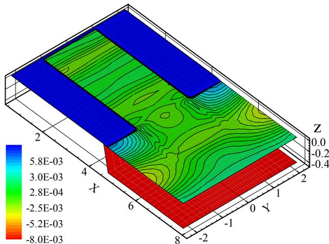
Fig. 8 Snapshot of free-surface elevation from linearly modeling results at  $t = 1800\text{s}$  for Case 3, i.e., the longitudinal bottom slope = 0.1 with incident wave frequency,  $f_1 = 0.55788\text{ Hz}$ .
