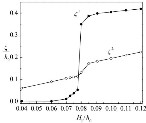
Fig. 6 Maximum amplitudes at the backwall within the harbor of slope  $s = 0.10$  for various incident heights but constant frequency  $f = 0.55788\text{Hz}$ : —●—, transverse oscillations ( $f^T = 0.27894\text{Hz}$ ); -○-, longitudinal oscillations ( $f^L = 0.55788\text{Hz}$ ).
