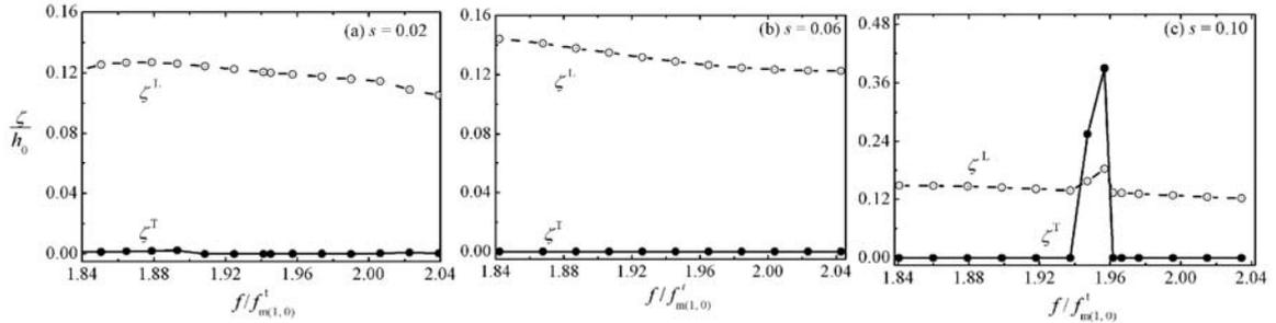
**Fig. 2** Maximum wave amplitudes at the backwall as a function of the incident wave frequency for subharmonic generations of transverse oscillations. —○— refers to longitudinal oscillation amplitude  $\zeta^L$ , and —●— refers to transverse oscillation amplitude  $\zeta^T$ ; Notice the resonance frequencies corresponding to mode  $(1, 0) f_{m(1,0)}^L$  for three cases are different (see Table 1).
