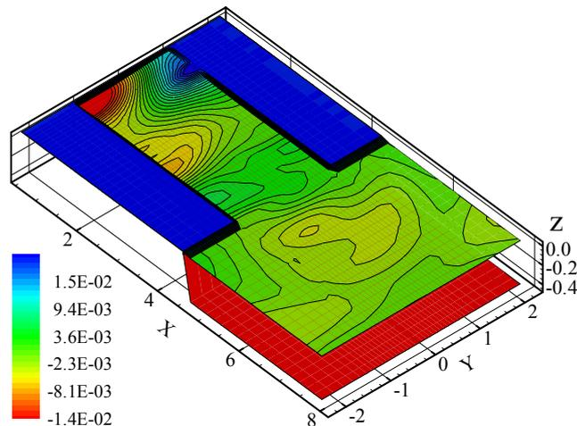
**Fig. 5 Snapshot of free-surface elevation from FUNWAVE modeling results at  $t = 1800\text{s}$  for Case 3, i.e., the longitudinal bottom slope = 0.1 with incident wave frequency,  $f_1 = 0.55788\text{ Hz}$ .**
