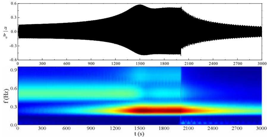
**Fig. 3** Surface elevations and corresponding wavelet amplitude spectrum for case 3 at the probe S1 with the incident frequency  $f = 0.55788\text{Hz}$ , which is the maximum amplified subharmonic frequency.
