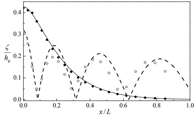
Fig. 4 Comparisons of oscillation profiles along the sidewall of the harbor induced by a monochromatic wave with frequency  $f = 0.55788\text{Hz}$  and wave height  $H_1 = 0.00454\text{m}$ :  $\bullet$ , transverse oscillations with frequency  $f^T = 0.27894\text{Hz}$ ;  $\circ$ , longitudinal oscillations with frequency  $f L = 0.55788\text{Hz}$ ; —, theory for transverse oscillations; ---, theory for longitudinal oscillations.
