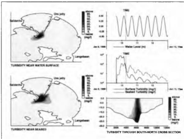
**Figure 5: Predicted turbidity plume 3 hours after a simulated failure of the dredge line has been repaired**
