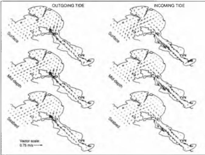
**Figure 4: Modelled currents in Saldanha Bay at neap tide with a 10 m/s SW wind**
